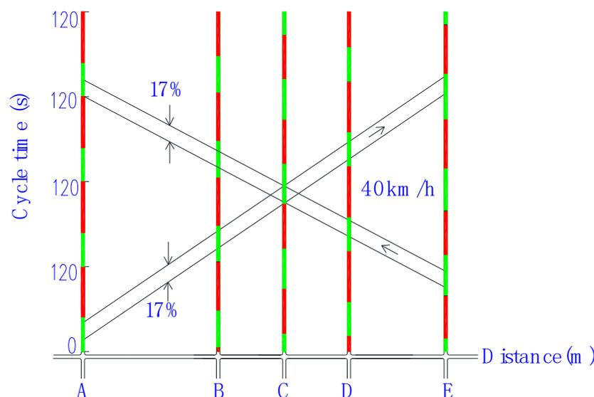
**Figure 3.** Bidirectional green wave design result under symmetric release mode. A~E represent the five adjacent intersections on Ziwu Road. The green bar indicates the green time of the coordinated phase. The red bar indicates the red time of the coordinated phase.
