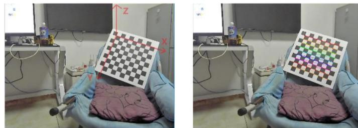
Figure 1. World coordinate system construction and corner detection.
