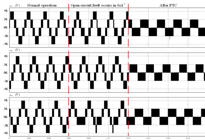
**Figure 19.** Output voltage with an open-circuit fault in  $S_{a1}^+$  after FTC.
