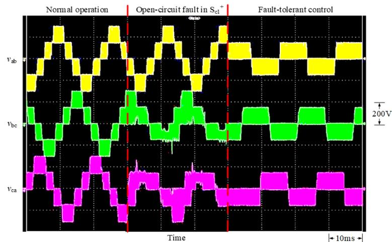
**Figure 24.** Measured waveform of the output voltage generated by the fault-tolerant control strategy when an open-circuit fault occurs in the switch  $S_{c1}^+$ .
