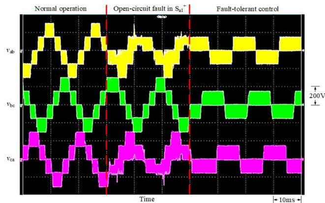
**Figure 22.** Measured waveform of the output voltage generated by the fault-tolerant control strategy when an open-circuit fault occurs in the switch  $S_{a1}^+$ .
