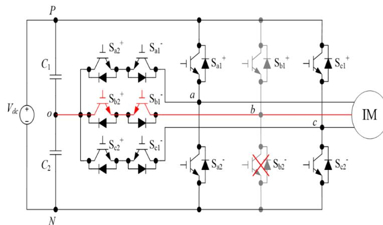
**Figure 15.** FTC for the occurrence of an open-circuit fault in  $S_{b2}^-$ .
