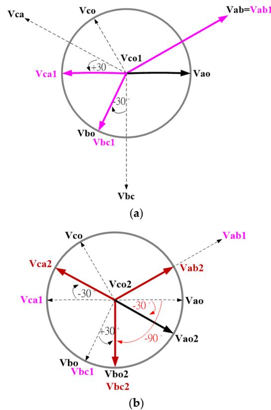
**Figure 18.** Voltage phasor diagram of the fault-tolerant control when a fault occurs in the switch  $S_{c1}^+$  or  $S_{c2}^-$ ; (a) unadjusted voltage phase angle; (b) adjusted phase angle of the  $a$ -phase voltage such that it is  $30^\circ$  behind that of the original phase angle of the  $a$ -phase voltage; adjusted phase angle of the  $b$ -phase voltage such that it is  $150^\circ$  behind the original phase angle of the  $a$ -phase voltage.
