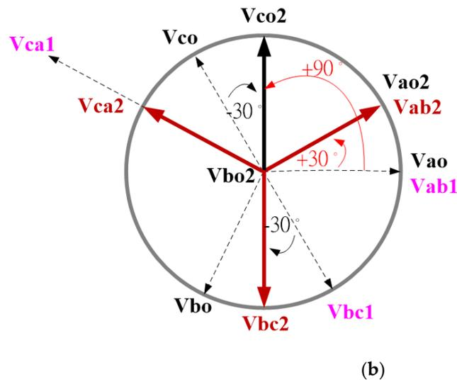
**Figure 16.** Voltage phasor diagram of fault-tolerant control when a fault occurs in the switch  $S_{b1}^+$  or  $S_{b2}^-$ ; (a) unadjusted voltage phase angle; (b) adjusted phase angle of the  $a$ -phase voltage such that it is  $30^\circ$  ahead of the original phase angle of the  $a$ -phase voltage; adjusted phase angle of the  $c$ -phase voltage such that it is  $90^\circ$  ahead of the original phase angle of the  $a$ -phase voltage.
