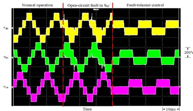
**Figure 23.** Measured waveform of the output voltage generated by the fault-tolerant control strategy when an open-circuit fault occurs in the switch  $S_{b2}^-$ .
