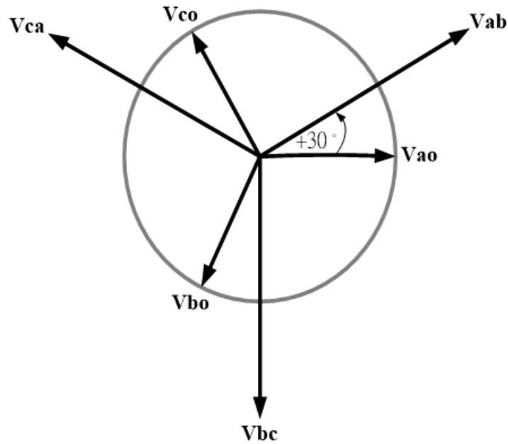
Figure 12. Balanced three-phase voltage phasor diagram of a switch without fault.
