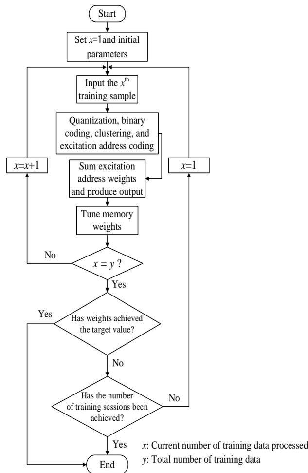
**Figure 11.** Training flowchart for the CMAC-based fault diagnosis system for inverters.
