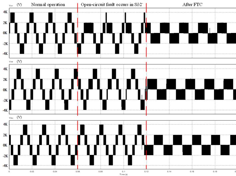
Figure 20. Output voltage with an open-circuit fault in  $S_{b2}^-$  after FTC.
