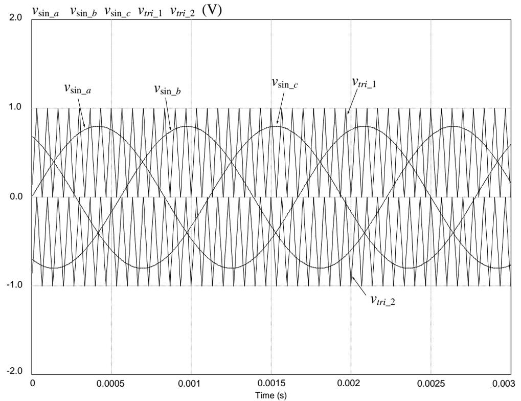
**Figure 3.** The time command PWM generation scheme of switches for a three–level T–type inverter.
