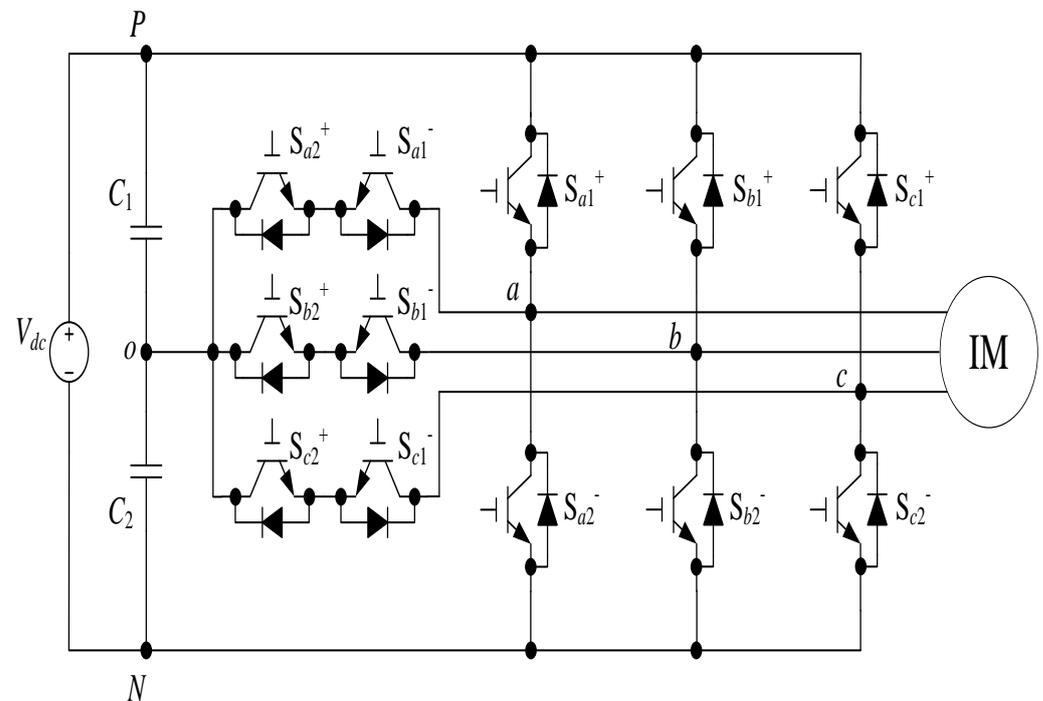
Figure 2. The three-level T-type inverter architecture.
