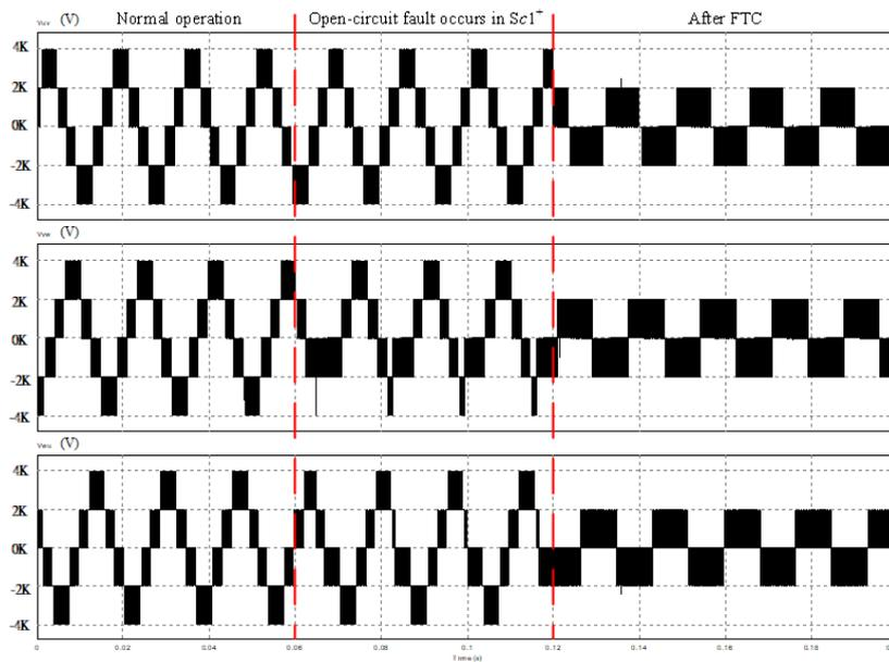
Figure 21. Output voltage with an open-circuit fault in  $S_{c1}^+$  after FTC.
