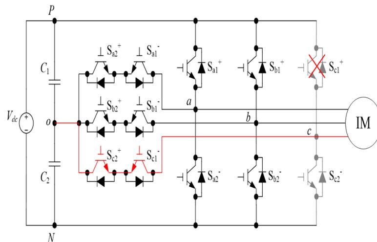
**Figure 17.** FTC for the occurrence of an open-circuit fault in  $S_{c1}^+$ .
