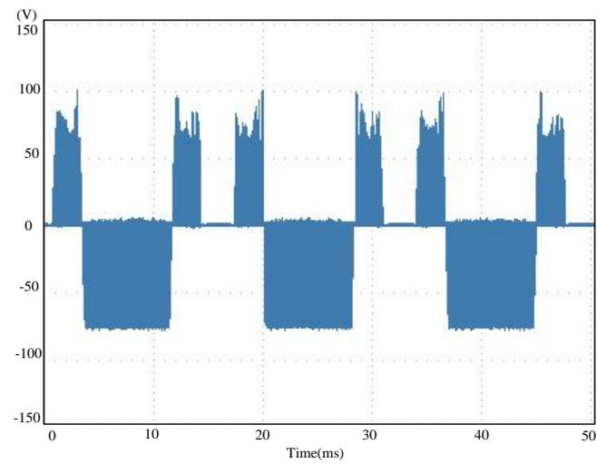
**Figure 6.** Waveform of the  $a$ -phase output voltage ( $v_{ao}$ ) of the inverter at a working frequency of 60 Hz with a fault in switch  $S_{a1}^+$ .
