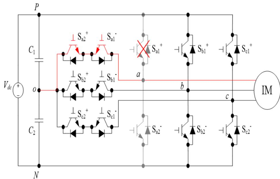
Figure 13. FTC for the occurrence of an open-circuit fault in  $S_{a1}^+$ .
