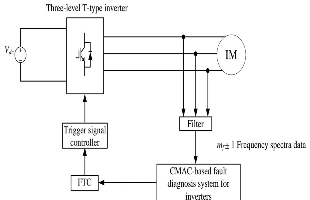
**Figure 1.** The CMAC-based fault diagnosis system for inverter architecture.
