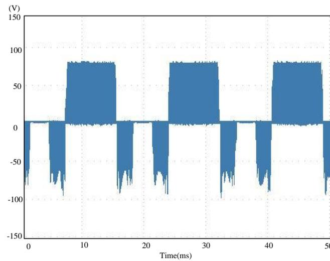
**Figure 7.** Waveform of the  $b$ -phase output voltage ( $v_{bo}$ ) of the inverter at a working frequency of 60 Hz with a fault in switch  $S_{b2}^-$ .
