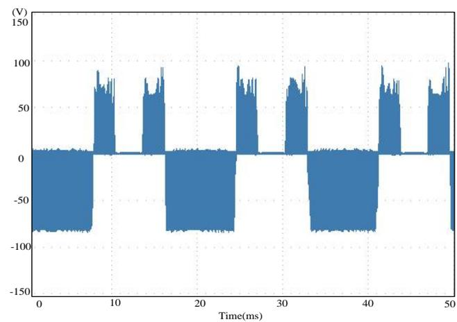
**Figure 8.** Waveform of the  $c$ -phase output voltage ( $v_{co}$ ) of the inverter at a working frequency of 60 Hz with a fault in switch  $S_{c1}^+$ .
