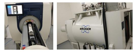
Figure 1. Photographs of Bruker's small animal 7 Tesla PET/MRI scanner.
