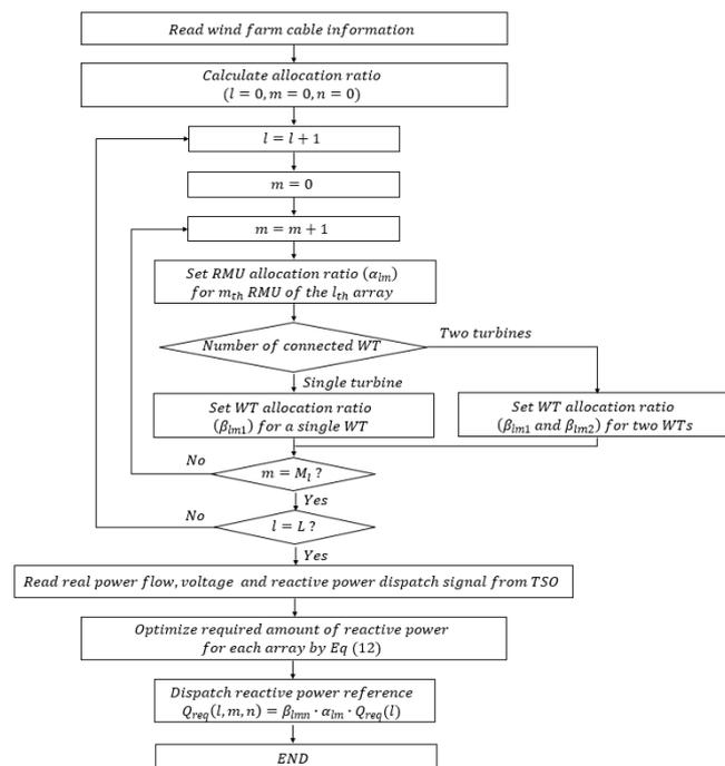
Figure 5. Flow chart of the reactive power allocation algorithm for the Dongbok wind farm.
