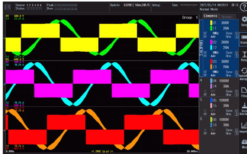
Figure 21. Exemplary waveforms of the three-phase TNPC converter output voltages and currents for rms value of the output current  $I_{Orms} = 11.0$  A and inductive reactive power generation.
