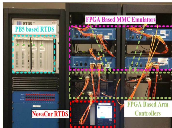
**Figure 10.** CHIL implementation set-up for MTDC grid.
