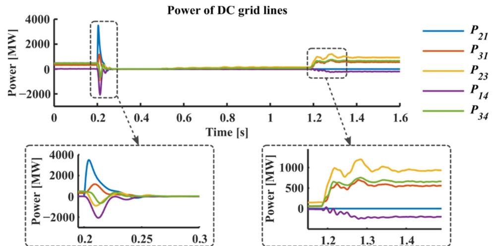
Figure 20. Power flow in the DC transmission lines with fault at location F3.
