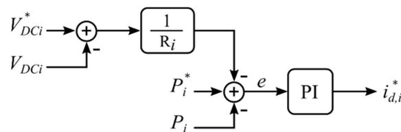
Figure 4. Droop control block diagram.
