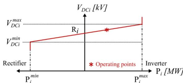
Figure 5. Droop control characteristics.
