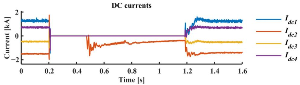
Figure 17. DC currents of the MTDC terminals with DC fault at location F2.
