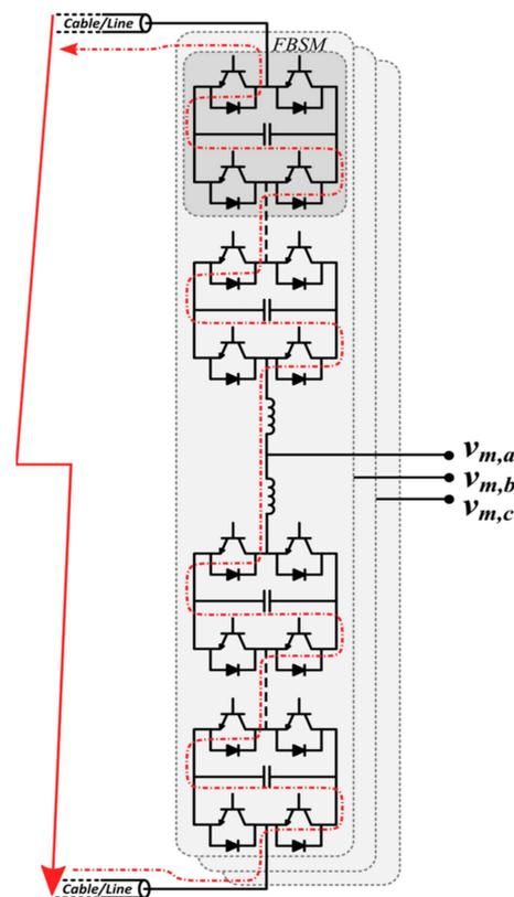
**Figure 7.** DC fault current flow in MMC-based FBSM circuits.
