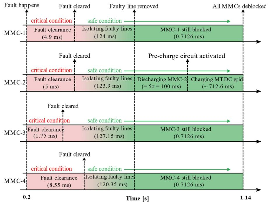
Figure 15. Fault clearance and restoration time of MMCs under DC fault at location F1.
