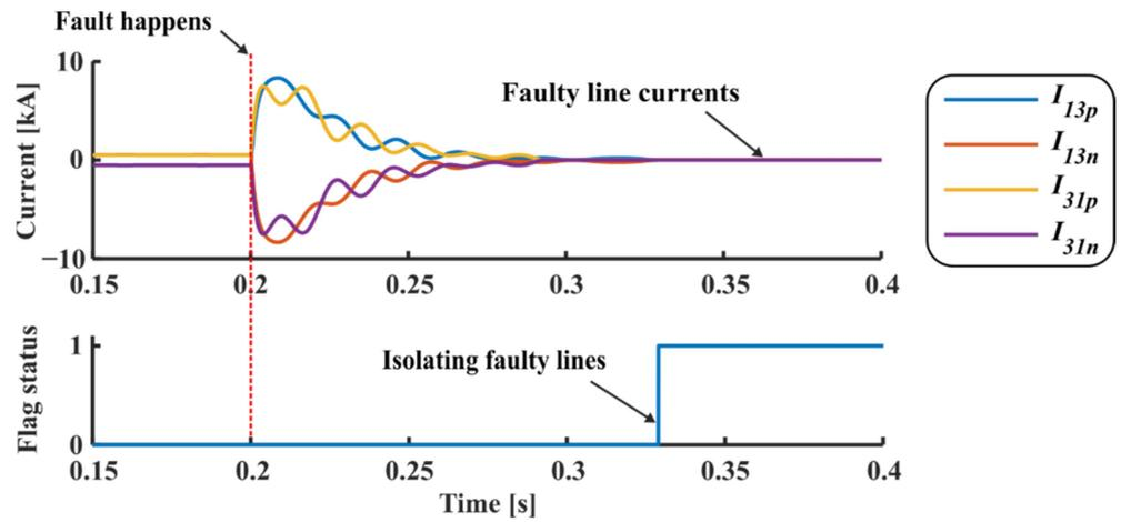
Figure 13. Fault currents and isolation status with DC fault at location F1.
