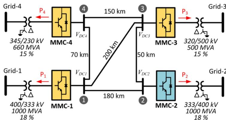
Figure 1. A mesh-connected four-terminal MMC system.
