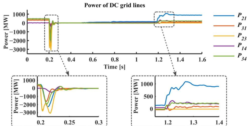
Figure 16. Power flow in the DC transmission lines with fault at location F2.
