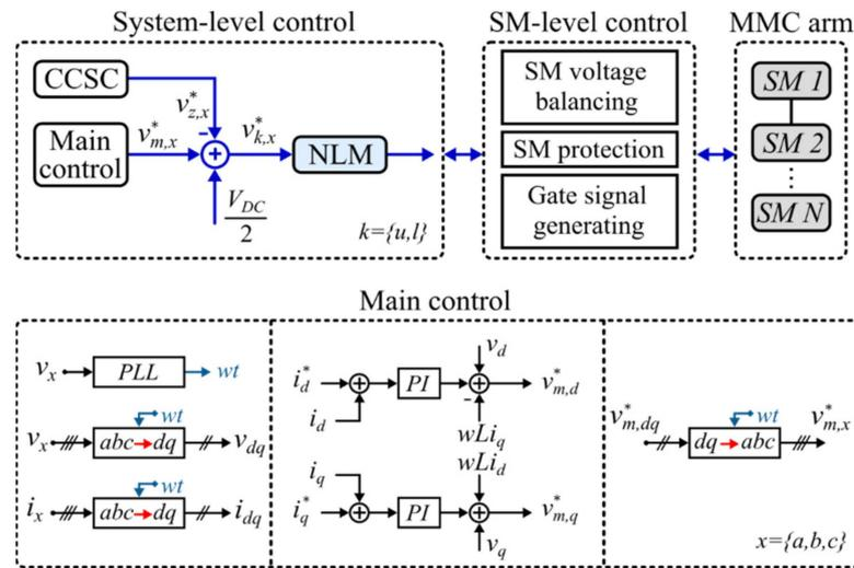
Figure 3. MMC control structure.
