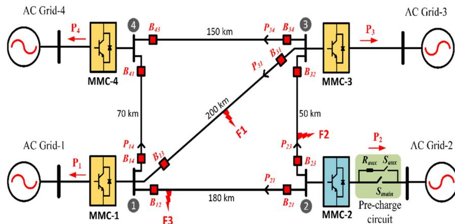
**Figure 11.** MMC-based MTDC system for the DC fault study.
