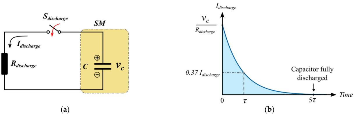
Figure 9. (a) Discharging system for single SM; (b) Capacitor discharging current.
