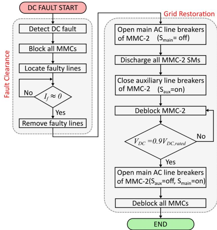
Figure 6. DC fault clearance and grid restoration flowchart.
