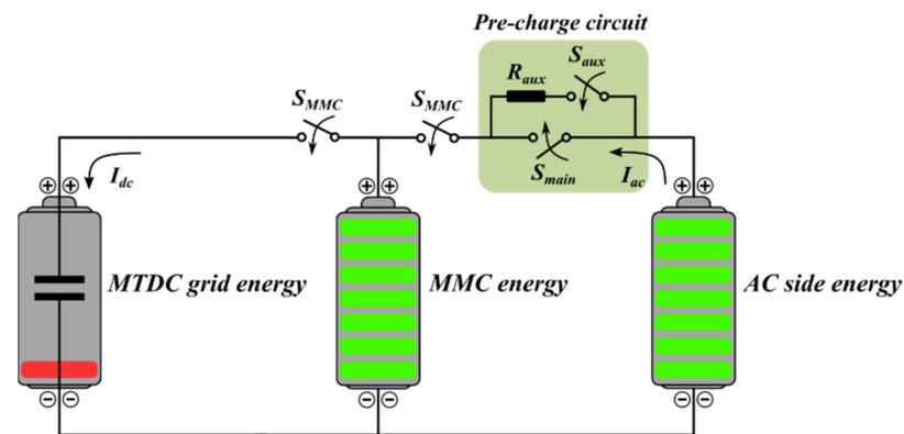
Figure 8. Simplified illustration of MTDC grid energy level after DC fault clearance.
