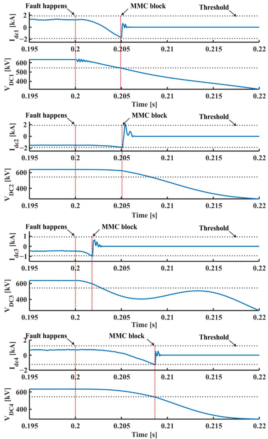
Figure 12. DC currents and voltages of MMCs with P2P DC fault at location F1.
