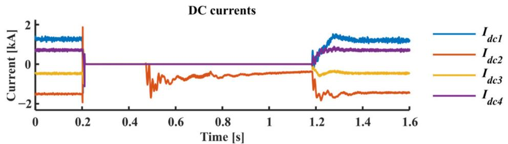
Figure 19. DC currents of the MTDC terminals with DC fault at location F3.
