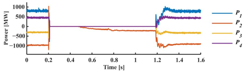
Figure 18. Net injected power  $P_i$  into the MMC terminals with DC fault at location F2.
