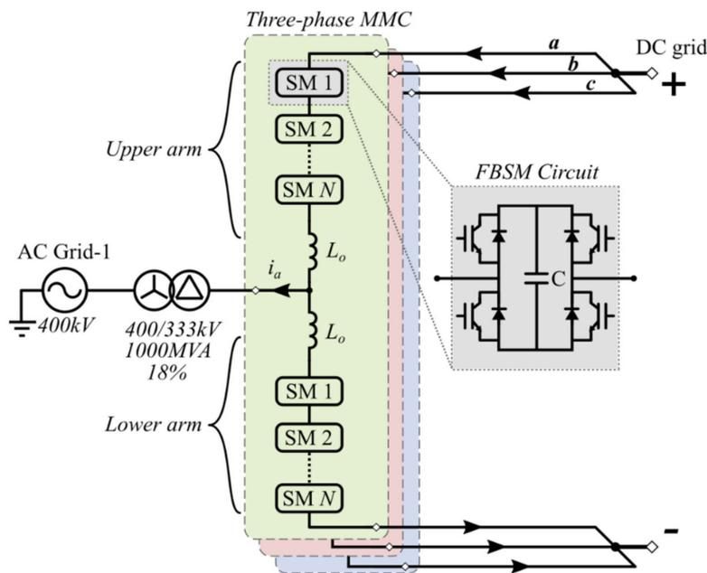
Figure 2. An FBSM structured three-phase MMC configuration (MMC-1).
