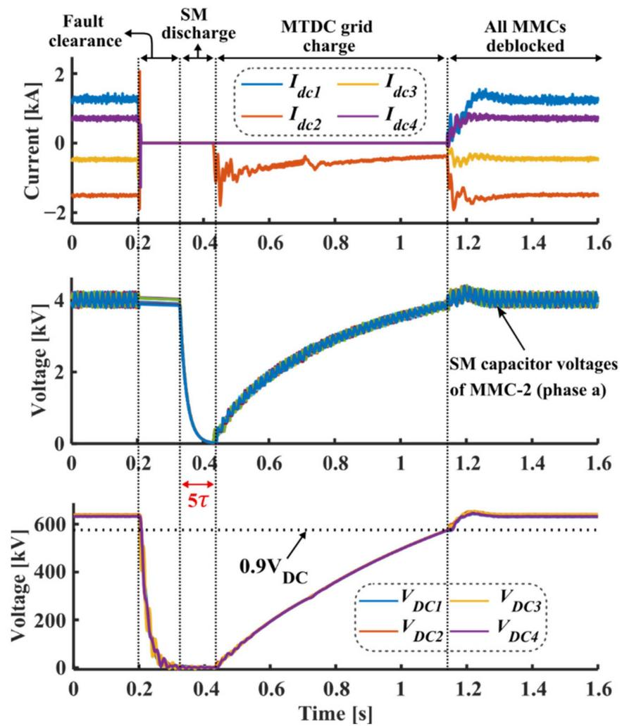
Figure 14. DC currents, voltages, and MMC-2 SM voltages with fault at location F1.
