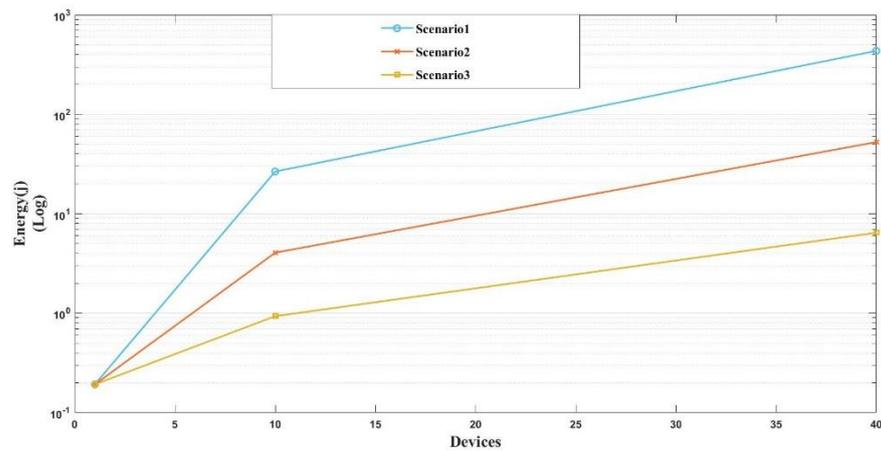
Figure 4. Energy consumption for nodes 1, 10, and 40—when distance is 200 m.
