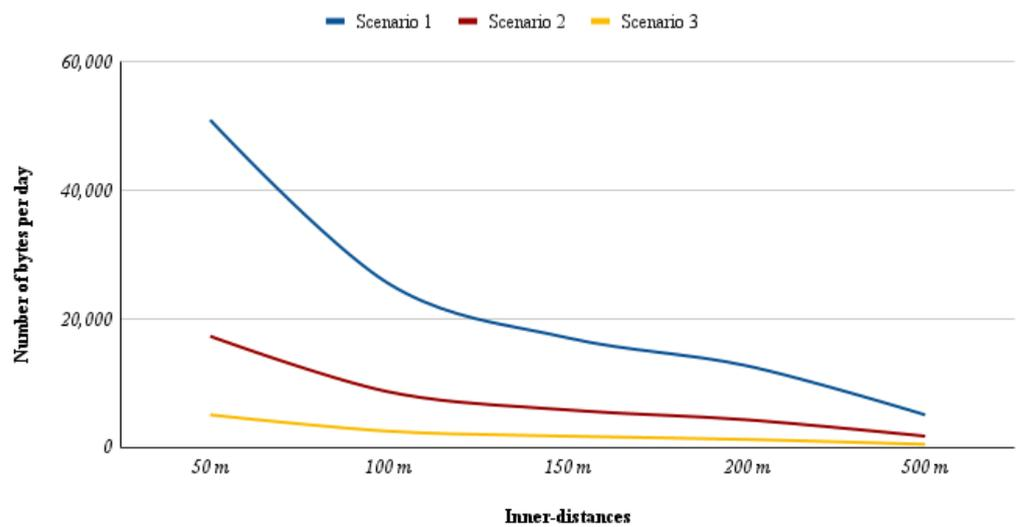
**Figure 3.** The number of bytes/days at different sensor distances (packet size is 255 bytes).
