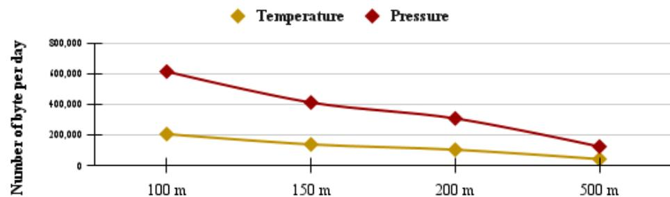
Figure 8. The number of bytes for temperature and pressure sensors at different distances.
