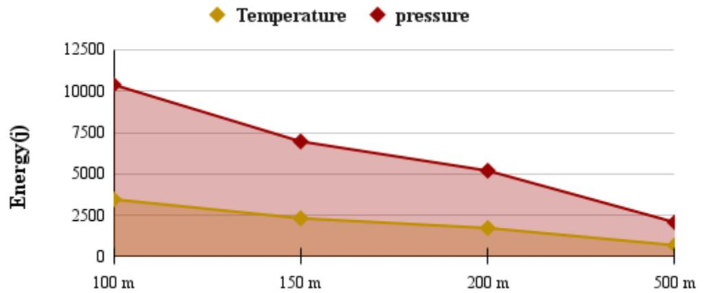
Figure 7. Energy for temperature and pressure sensors at different distances.
