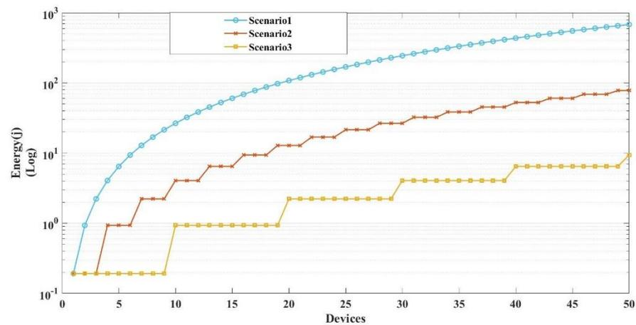
Figure 5. Energy consumption for the 50 devices—where the distance is 200 m.
