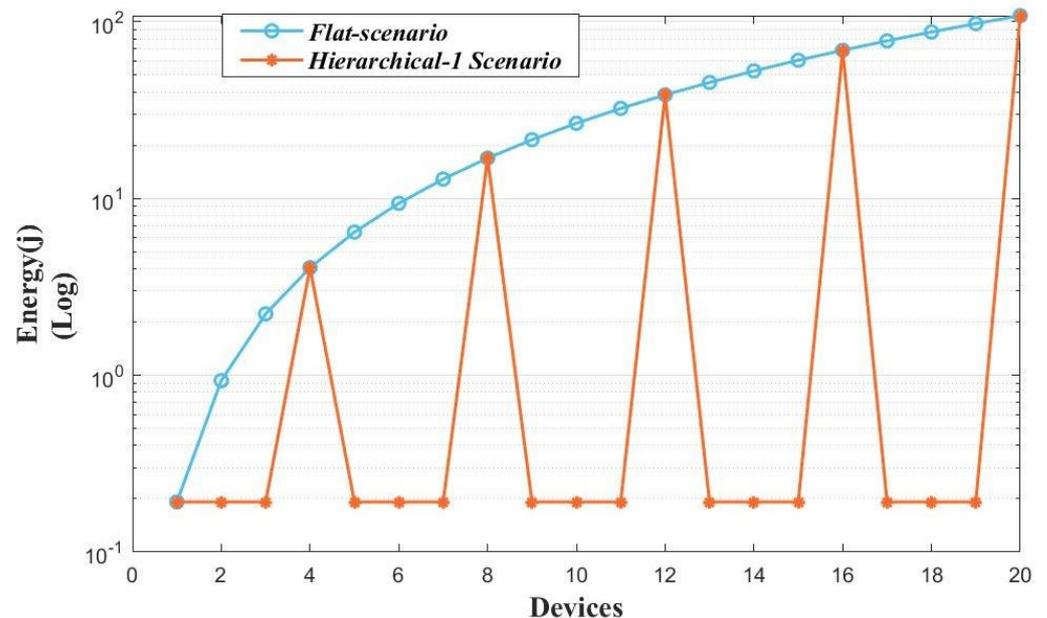
Figure 11. Energy consumption for simple sensors in different topologies.
