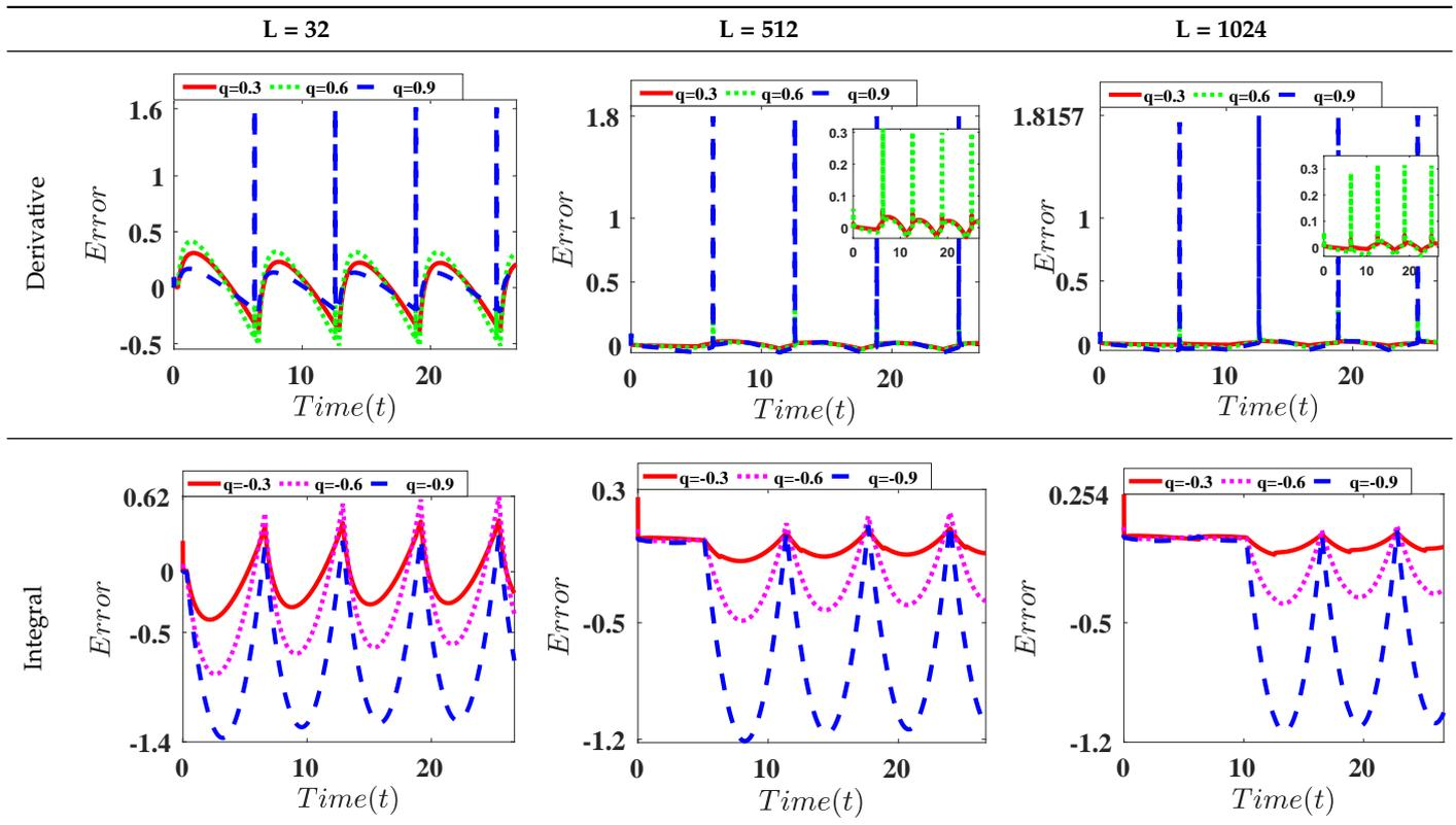
**Table 4.** The error of the proposed design results (differentiator and integrator) for a triangle signal input with respect to MATLAB results.
