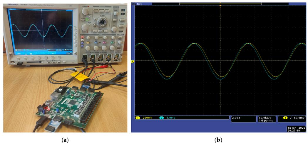
**Figure 4.** Oscilloscope FPGA results of integration process at  $q = -0.9$  and  $L = 20$  for a sine signal as input; (a) FPGA testing environment, (b) proposed approach response.
