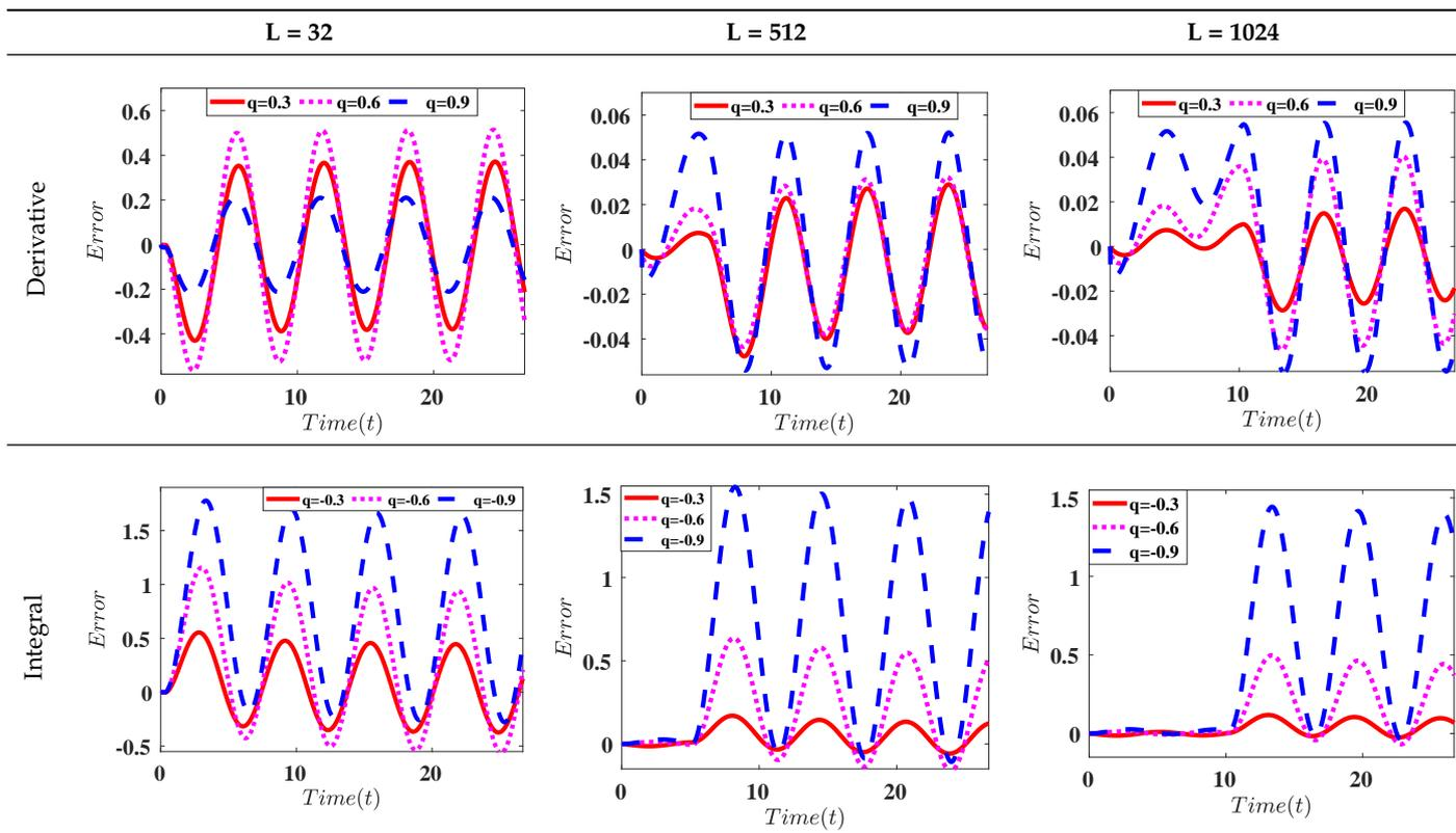
**Table 3.** The error of the proposed design results (differentiator and integrator) for a sawtooth signal input with respect to MATLAB results.
