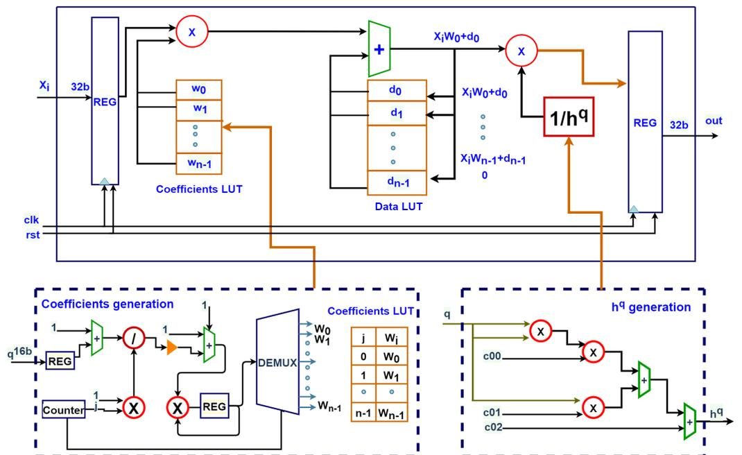
**Figure 2.** The hardware architecture of the proposed approach for the integrator and differentiator GL operator.
