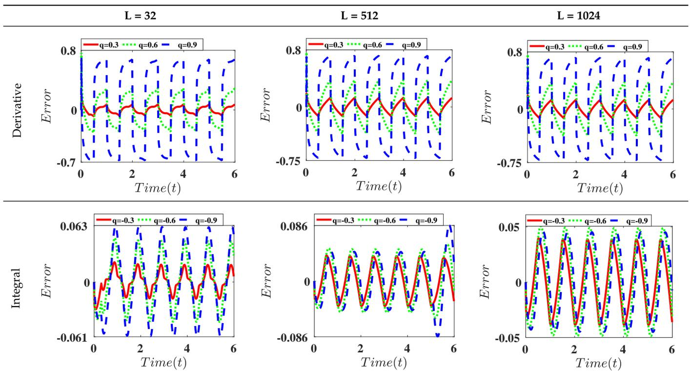
**Table 5.** Comparison between the maximum errors of the proposed implementation and [29] for sine signal.
