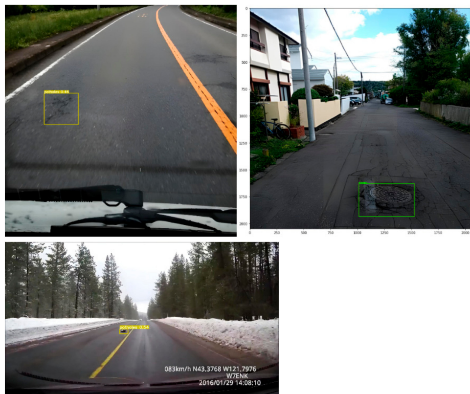
Figure 7. Misclassifications experienced during validation, where a manhole cover, crack, and black nylon are classified as pothole instance.
