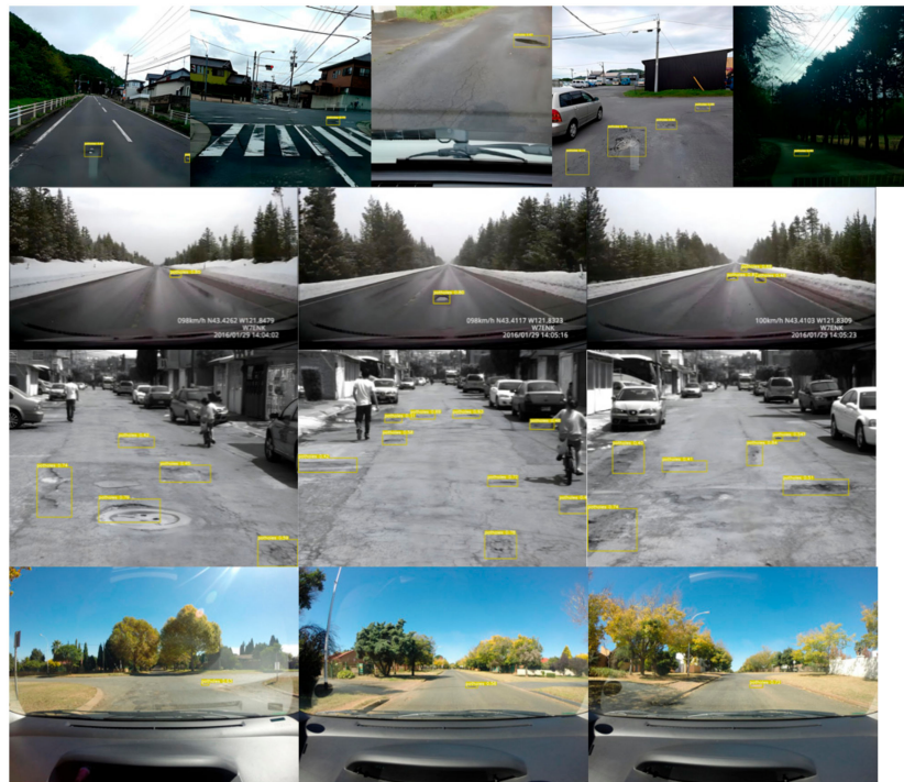
Figure 6. Detected potholes from the validation set using the ESRGAN + YOLOv5 method, with each row showing images from the different datasets.
