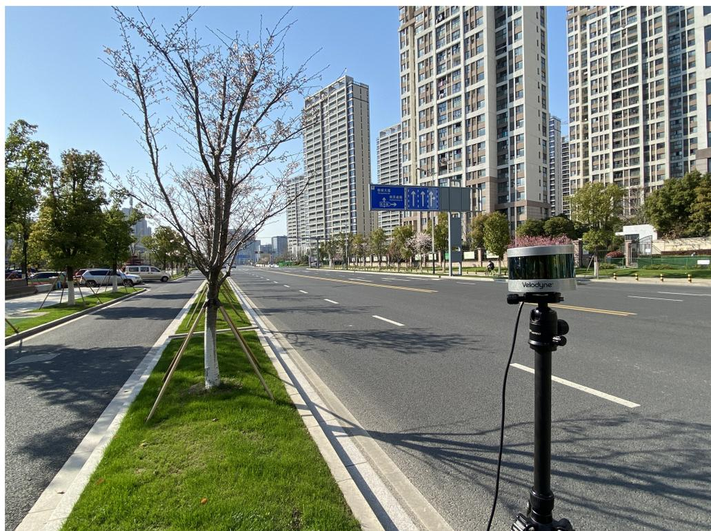
Figure 1. Roadside LiDAR and traffic sign.
