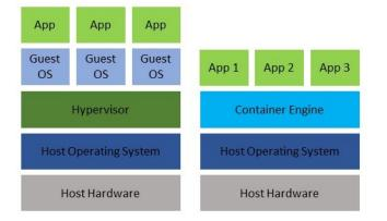
Figure 3. Full System Virtualisation and Container Architectures.
