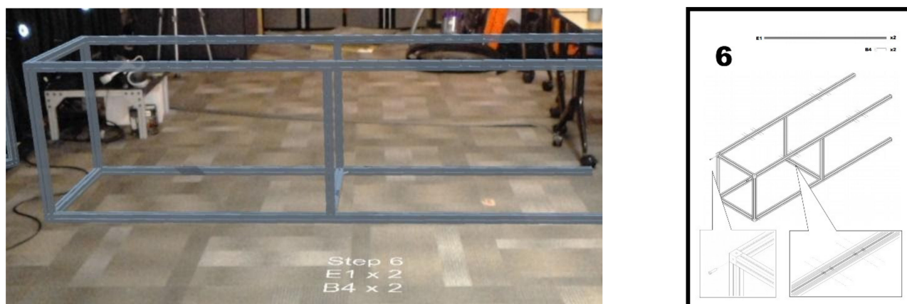
Figure 7. Step 6 of the Destiny construction manual depicted in the HoloLens on the left, and as a traditional orthographic drawing on the right.
