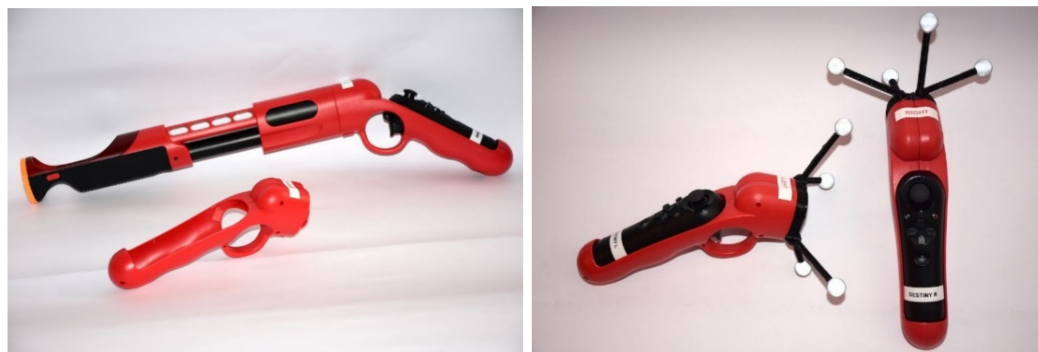
Figure 10. To the left is the dreamGEAR PS3 Move Equalizer shotgun holster. On the right are the Destiny controllers which have replaced the barrel portion with a 3D printed tracking constellation.
