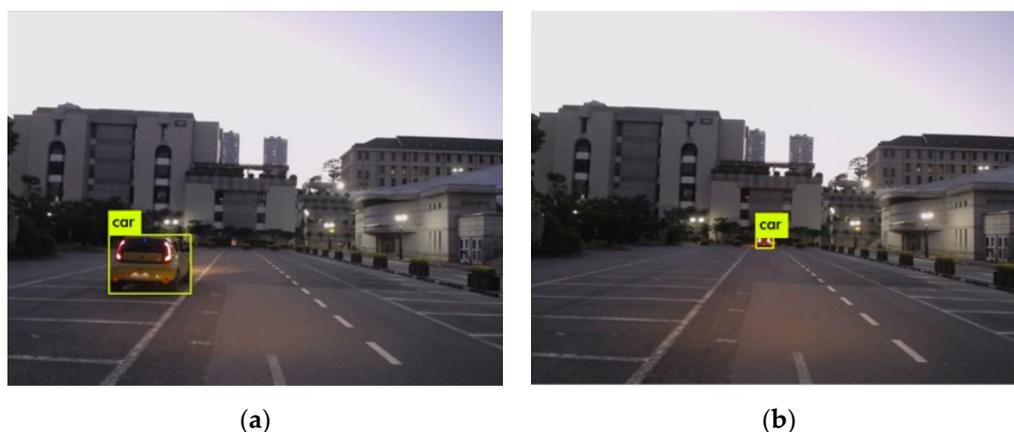
**Figure 3.** (a) The bounding box of the SV in the adjacent lane and close up; (b) the bounding box of the SV in the same lane and far away.
