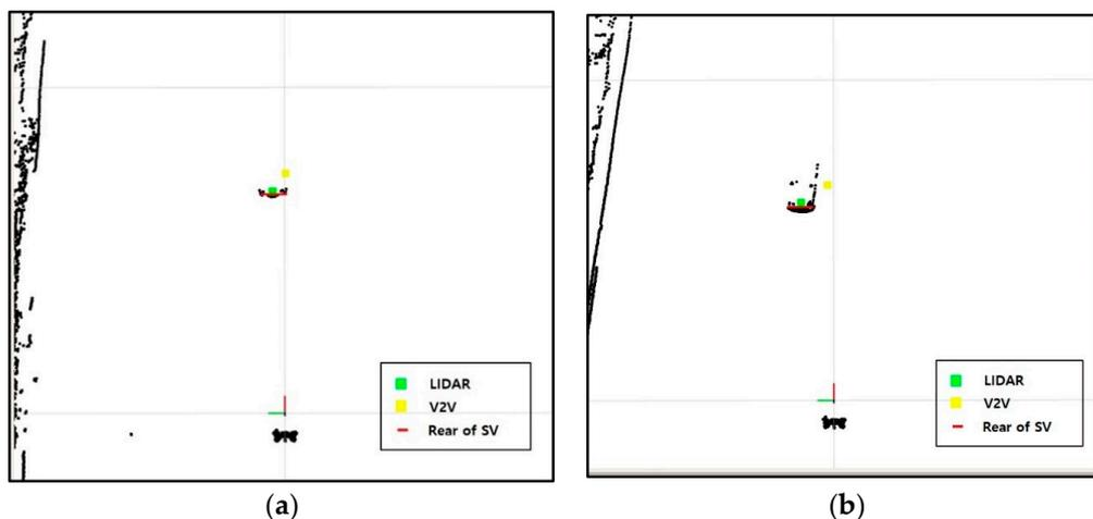
**Figure 4.** (a) In the case of keeping the lane in the same lane, Estimated location using V2V communications and LIDAR; (b) In the case of changing the lane in the adjacent lane, Estimated location using V2V communications and LIDAR.
