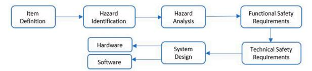
Figure 14. Functional safety process diagram.
