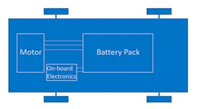
Figure 9. Layout of an electric drivetrain of an EV. Redrawn from [89].
