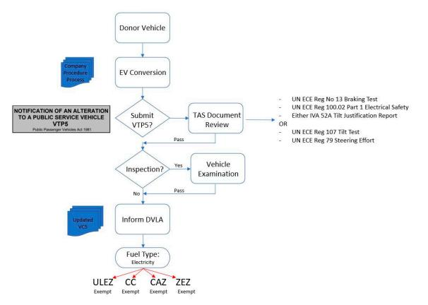
Figure 13. Schematic highlighting the apparent process of converting a bus to a fuel type of 'electricity'. CC: Congestion charge.
