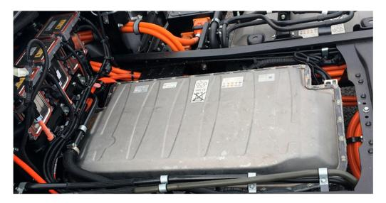
**Figure 16.** Chassis layout of a Mitsubishi Fuso E-canter, highlighting a sealed battery pack and organised orange HV cabling. Photo taken by the author.
