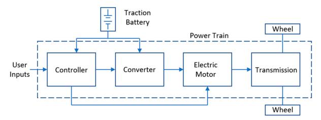
Figure 7. Block diagram highlighting the key components of an electric powertrain, redrawn from [48].
