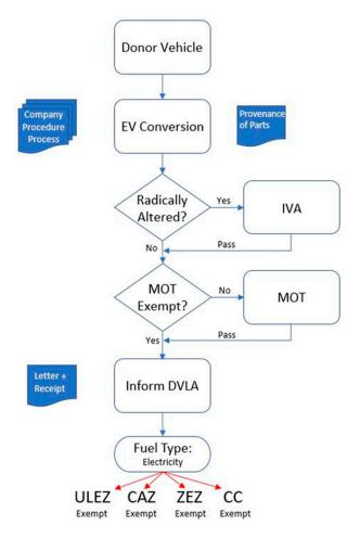
**Figure 12.** Schematic highlighting the apparent process of converting a car or van to a fuel type of 'electricity'. CC: Congestion charge.
