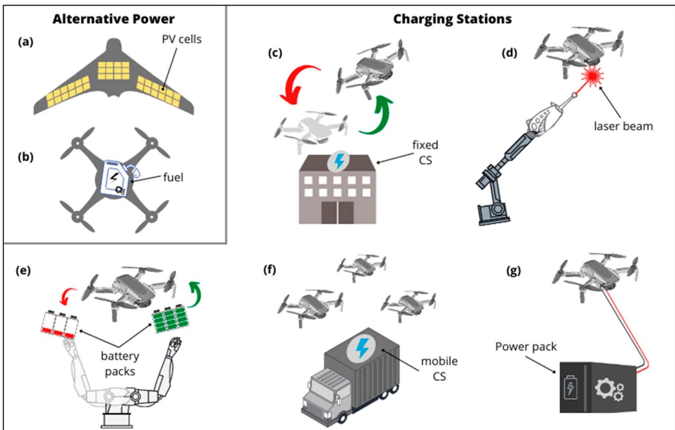
**Figure 1.** Drone power management. (a) Solar-powered drones, suitable for fixed-wing UAVs. (b) Hybrid-powered drones, combining energy from electric and fuel cells. (c) Drone-swapping method, with a fixed charging station. (d) Laser-powered on-the-air recharging. (e) Battery hot-swapping, without powering down the drone. (f) Mobile recharging stations, with programmed charging scheduling, and (g) Tethered drones.
