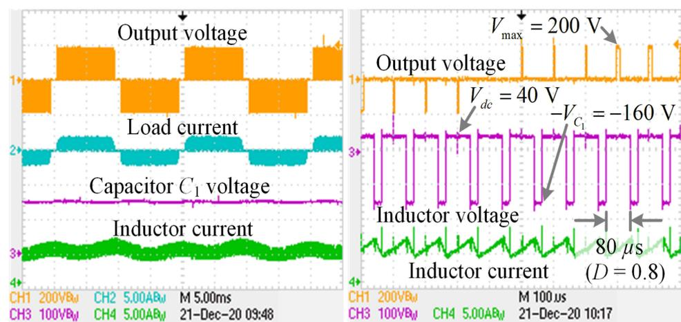
**Figure 7.** Experimental results of a single ICHB (3L),  $n = 1$ .
