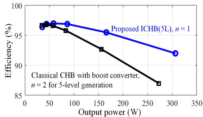
**Figure 6.** Efficiency of the proposed ICHB (5L) and comparison with the classical CHB for 5-level generation.
