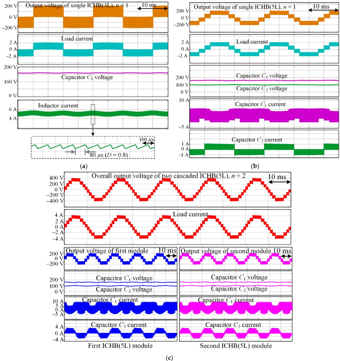
**Figure 5.** Simulation results of the proposed improved CHB multilevel inverters: (a) single module of 3-level topology (ICHB (3L),  $n = 1$ ), (b) single module of 5-level topology (ICHB (5L),  $n = 1$ ), and (c) two cascaded modules of 5-level topology (ICHB (5L),  $n = 2$ ).
