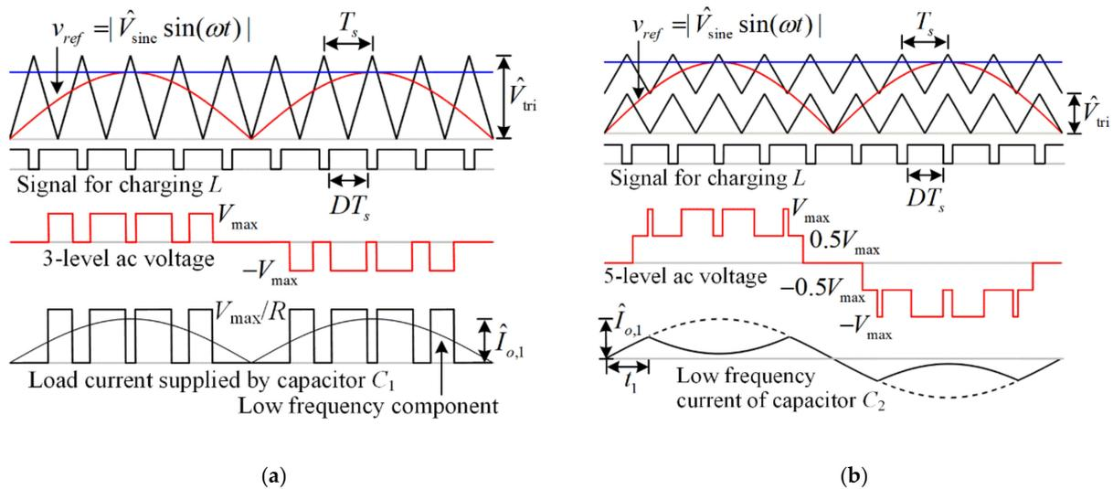
Figure 3. Pulse-width modulation scheme for the proposed topologies: (a) ICHB (3L) and (b) ICHB (5L).
