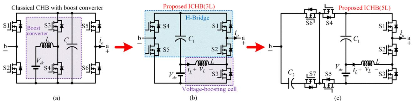
**Figure 1.** Derivation of the proposed ICHB topologies: (a) classical CHB with a front-end boost converter, (b) proposed ICHB (3L), and (c) proposed ICHB (5L).
