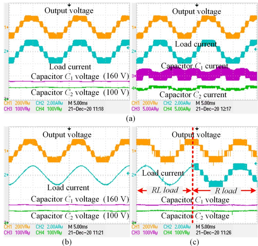
**Figure 8.** Experimental results of a single ICHB (5L),  $n = 1$ : (a) steady-state response under purely resistive  $R$  load, (b) steady-state response under series resistive-inductive  $RL$  load, and (c) transient response.
