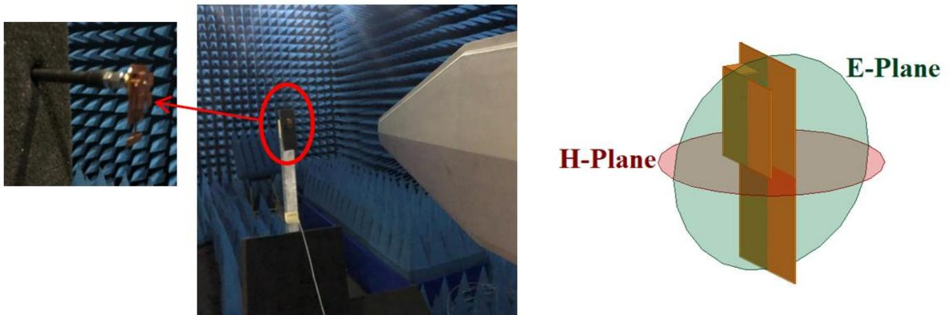
**Figure 12.** Measurement setup for PIFA gain measurements (anechoic chamber at the Microwave Laboratory of the University of Calabria) along with the definition of the E and H planes.
