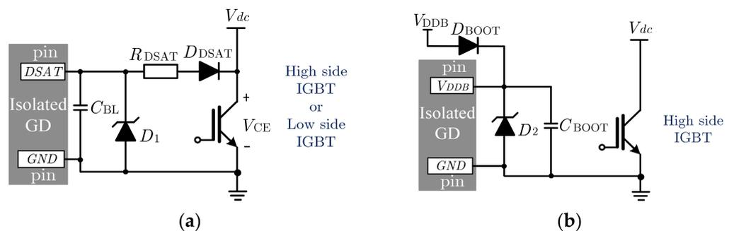
Figure 8. (a) Desaturation circuit; (b) Bootstrap.
