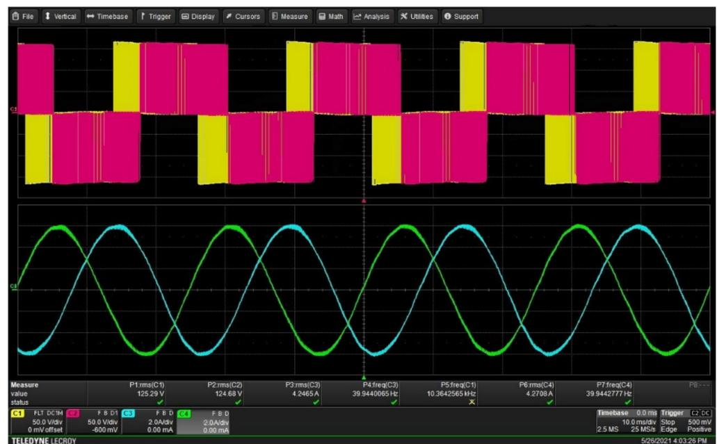
**Figure 16.** Experimental results of voltage and current at the output of the modular three-phase VSI, steady state (50 V/div, 2 A/div, 10 ms/div).
