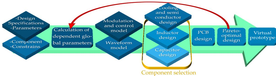
**Figure 5.** Simplified workflow of the virtual prototyping routine of the MODO-based process.
