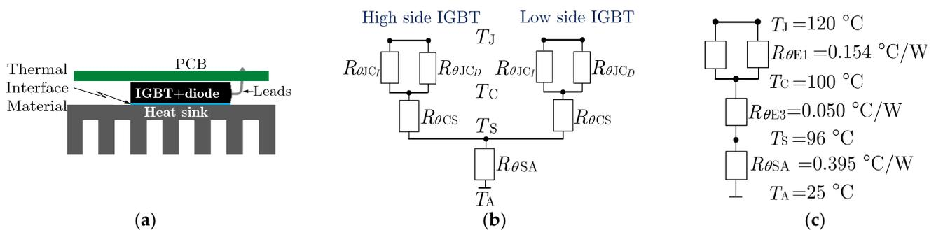
Figure 10. (a) IGBT+diode on the heat sink; (b) thermal resistance circuit and (c) parameters of the thermal circuit.
