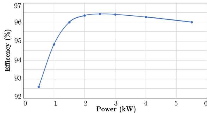
**Figure 18.** Efficiency curve of the power stage of a FB VSI for an input voltage of 180 V in DC-link.
