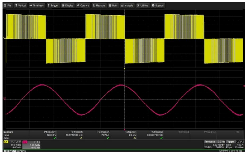
**Figure 15.** Experimental results of voltage and current at the output of the modular single-phase VSI, steady state (50 V/div, 5 A/div, 5 ms/div).
