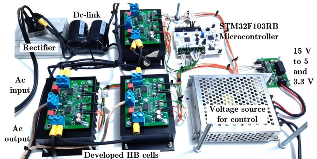
Figure 13. Photograph of the experimental setup.
