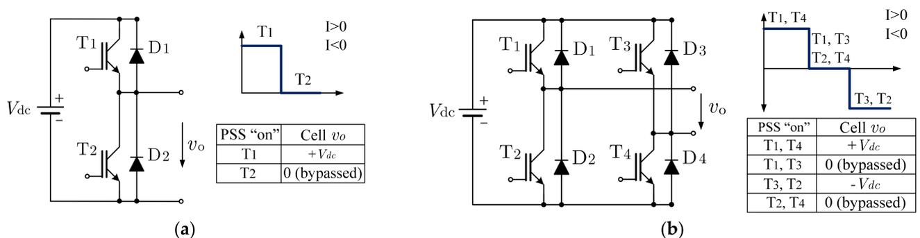
Figure 1. The most common power cells and their voltage levels: (a) HB cell; (b) FB cell.
