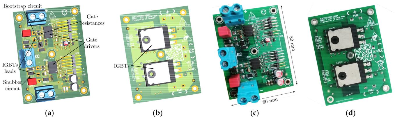
**Figure 11.** Developed HB cell: (a) 3D model, top view; (b) 3D model, bottom view; (c) implemented prototype, top view; (d) implemented prototype, bottom view.
