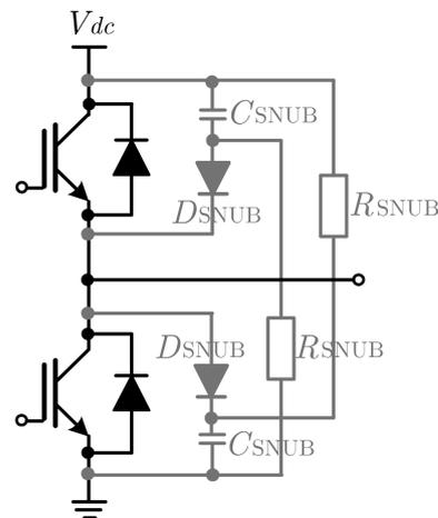
Figure 9. Discharge-suppressing RCD snubber circuit.
