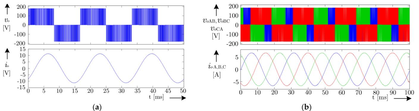
**Figure 12.** Simulated results of voltage and load current at the output of the inverter with open loop SPWM and in steady state; (a) single-phase FB VSI; (b) three-phase VSI.
