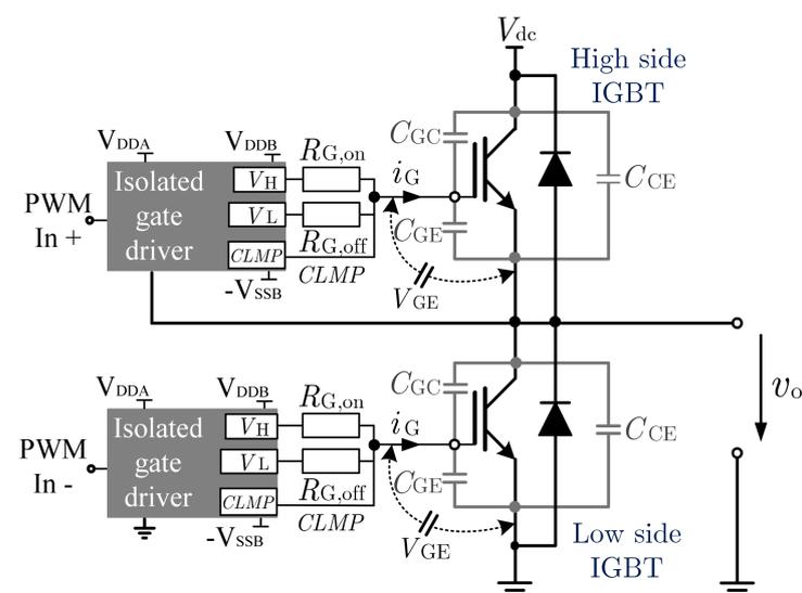
**Figure 7.** HB cell with basic push-pull resistive gate drives and parasitic capacitances of the IGBTs.
