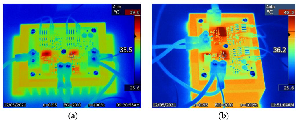
**Figure 17.** Temperature distribution of an HB cell with 50% of the nominal load: (a) after 30 min of operation; (b) after 3 h of operation.
