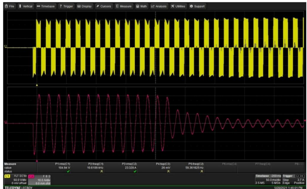
**Figure 14.** Experimental results of voltage and current at the output of the modular single-phase FB VSI, in dynamic state (50 V/div, 10 A/div, 50 ms/div).
