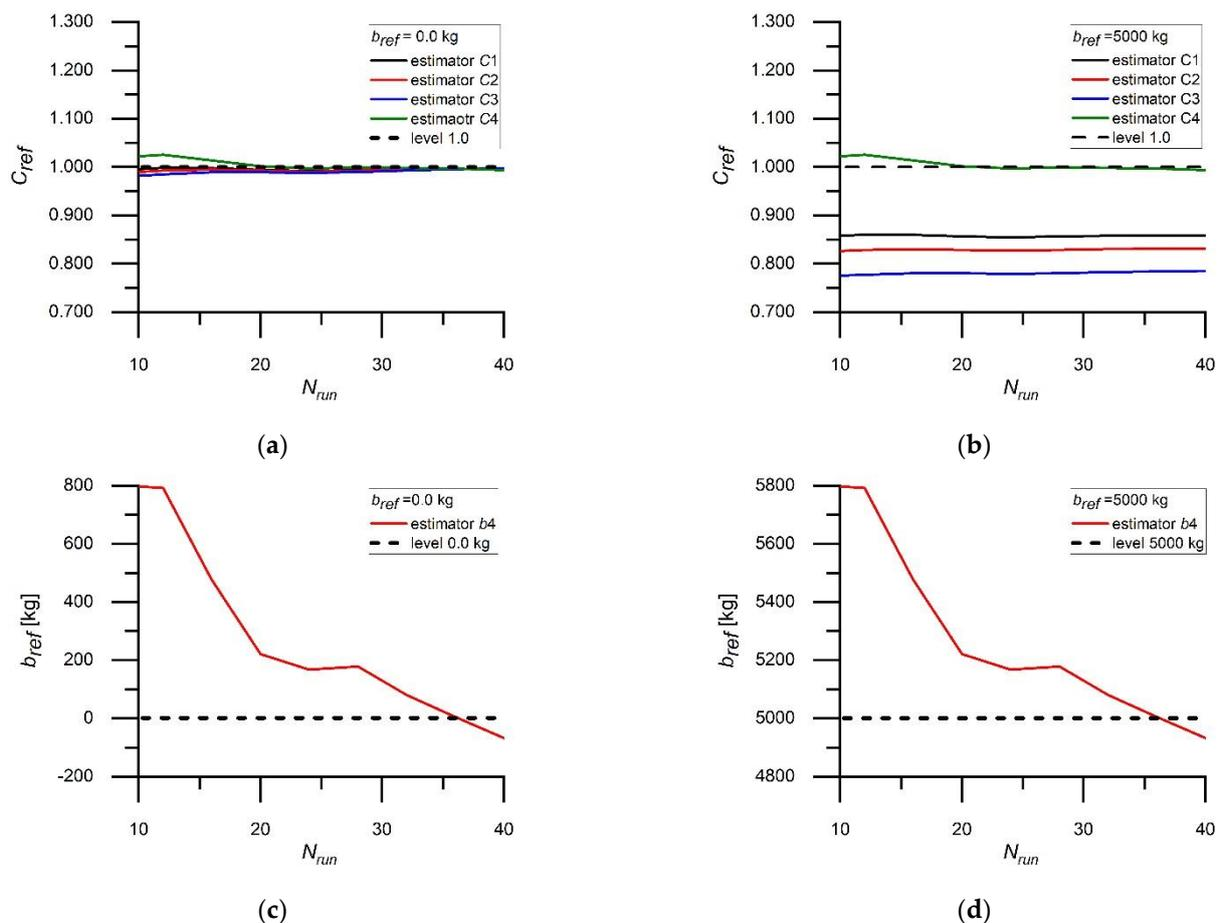
**Figure 8.** Estimation of the calibration coefficients (a,b)— $C_{ref}$ ; (c,d)— $b_{ref}$ , obtained using different estimators, respectively, for  $b_{ref} = 0$  kg and  $b_{ref} = 5000$  kg, as a function of the number of test vehicle runs  $N_{run}$ .
