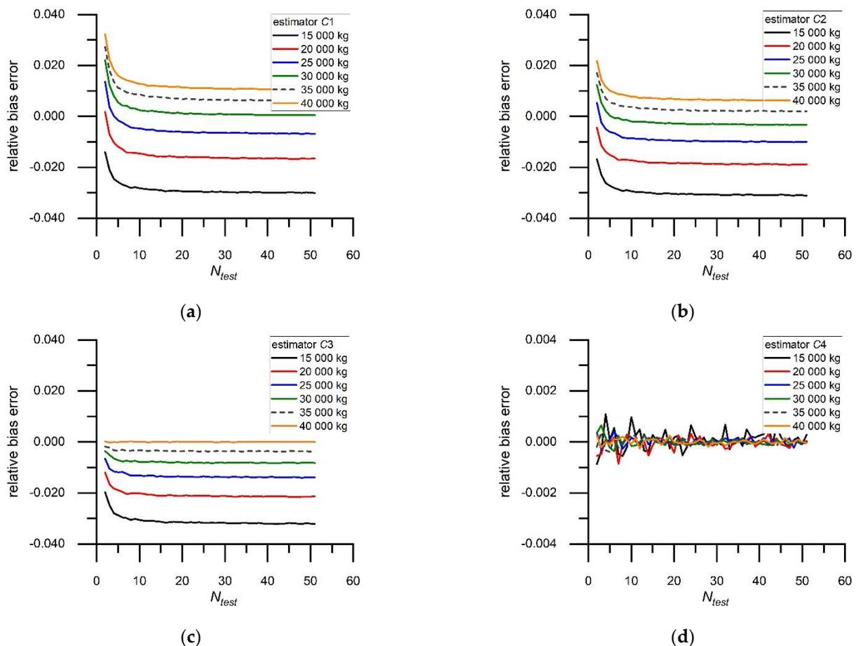
**Figure 5.** Influence of the weight distribution of test vehicles in the measurement range of the WIM system on the bias error of vehicle weighing results for various algorithms for estimating calibration coefficients ( $C_{ref} = 1$ ,  $b_{ref} = 0.1Z_{min}$ ). (a) estimator C1, (b) estimator C2, (c) estimator C3, (d) estimator C4.
