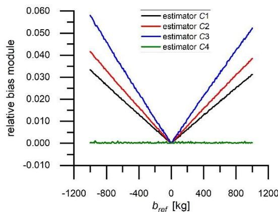
**Figure 1.** Effect of the shift  $b_{ref}$  of the WIM static characteristic on the relative bias error of the estimates of the C calibration factor for different calibration algorithms and  $C_{ref} = 1$ .
