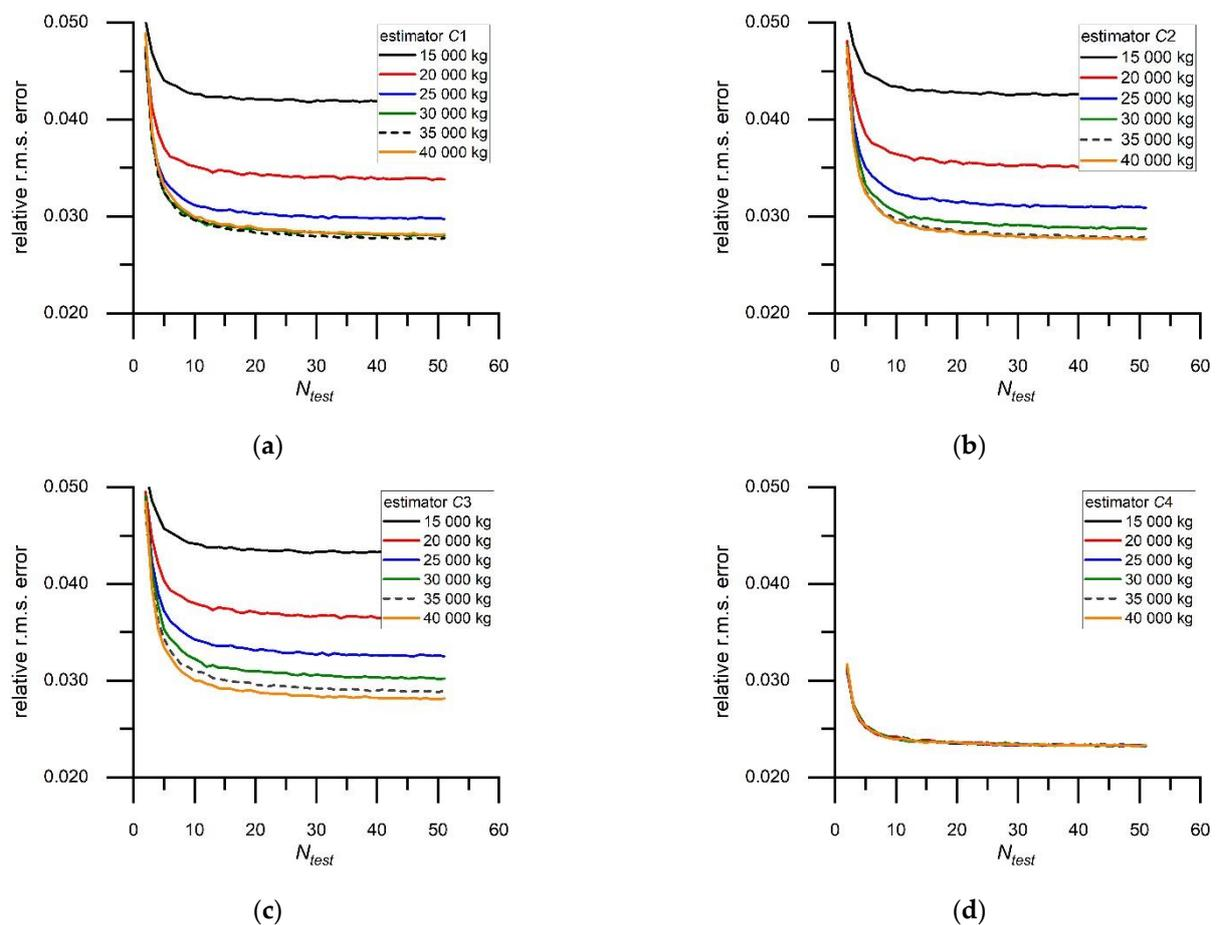
**Figure 4.** Influence of the weight distribution of test vehicles in the measurement range of the WIM system on the rms error of vehicle weighing results for various estimators of calibration coefficients ( $C_{ref} = 1$ ,  $b_{ref} = 0.1Z_{min}$ ), (a) estimator C1, (b) estimator C2, (c) estimator C3, (d) estimator C4.
