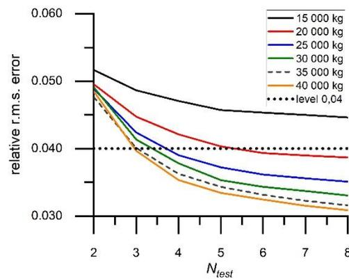
**Figure 6.** Illustration of the method for selecting parameters of the calibration process for the assumed, permissible error of weighing.
