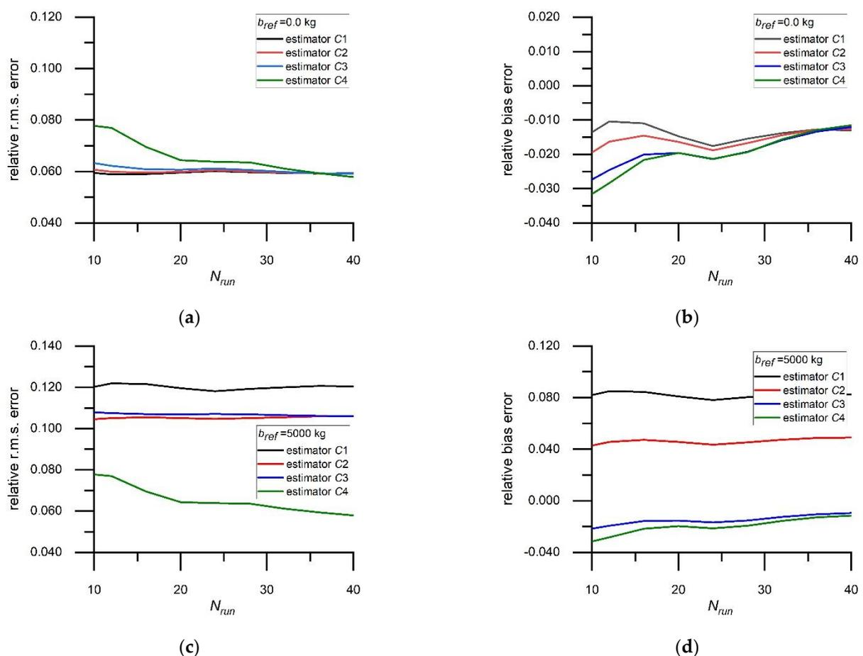
**Figure 7.** Dependence of weighing errors for the WIM system calibrated according to four discussing estimators on the number of runs of test vehicles  $N_{run}$ , respectively for (a,b)  $b_{ref} = 0$  kg and (c,d)  $b_{ref} = 5000$  kg.
