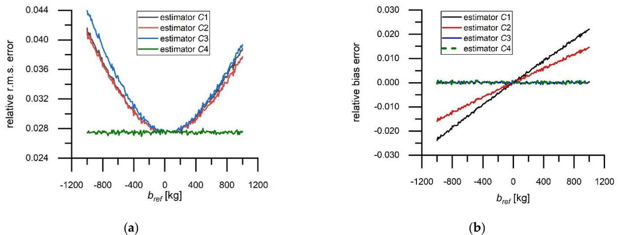
**Figure 2.** Influence of the WIM static characteristic shift on: (a) relative r.m.s. errors and (b) relative bias error of weighing,  $C_{ref} = 1$ .
