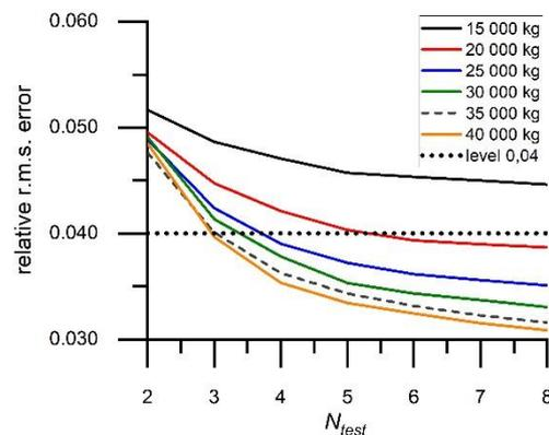
**Figure 6.** Illustration of the method for selecting parameters of the calibration process for the assumed, permissible error of weighing.
