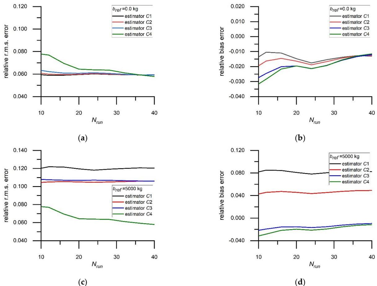
**Figure 7.** Dependence of weighing errors for the WIM system calibrated according to four discussing estimators on the number of runs of test vehicles  $N_{run}$ , respectively for (a,b)  $b_{ref} = 0$  kg and (c,d)  $b_{ref} = 5000$  kg.
