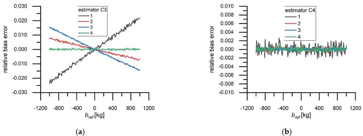
**Figure 3.** Bias of results of weighing on the WIM station calibrated according to the algorithm: (a) C3, (b) C4. (1–3) bias errors of weighing of three exemplary test vehicles and (4) sum of these bias errors,  $C_{ref} = 1$ .
