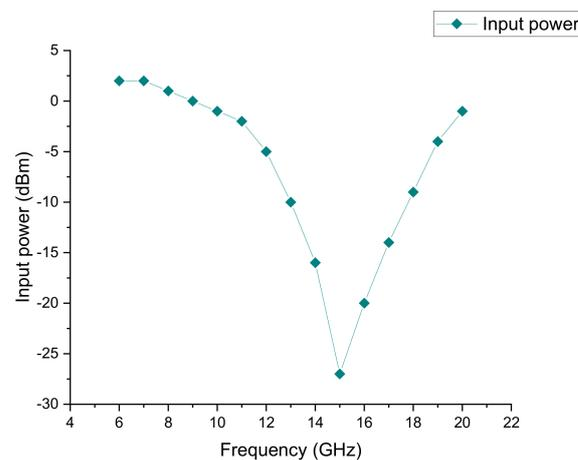
Figure 12. Measured simulated input sensitivity curves of the programmable frequency divider.
