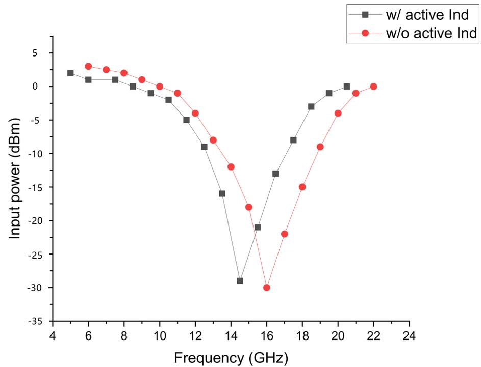
Figure 6. Simulated input sensitivity curves with and without active-inductor-based SCL DFFs.
