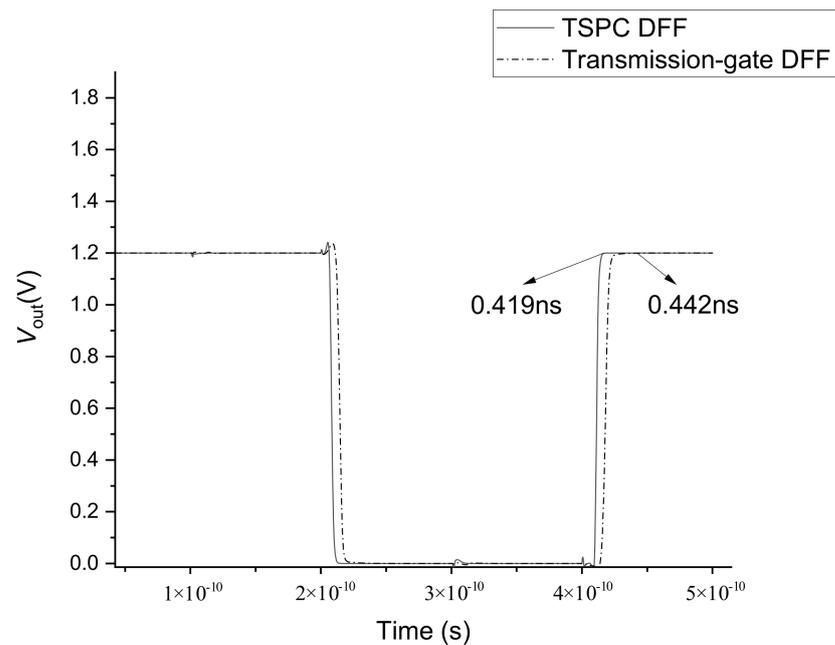
Figure 7. Simulated time delay of asynchronous divide-by-2 circuits based on different kinds of DFFs.
