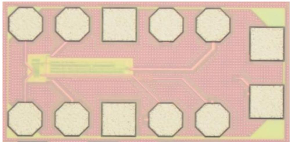
**Figure 9.** Chip microphotograph of the programmable frequency divider.
