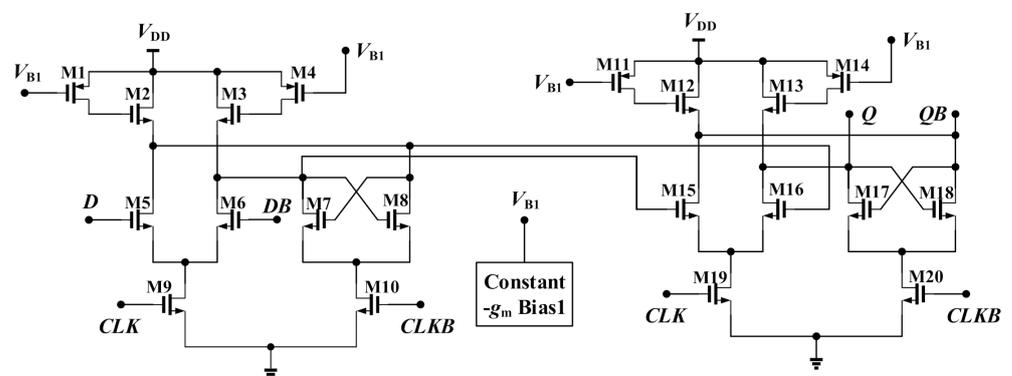
Figure 3. Schematic of the modified DFF based on active inductors.
