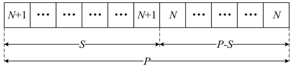
Figure 2. Working principle illustration for the frequency division ratio of the improved programmable frequency divider.
