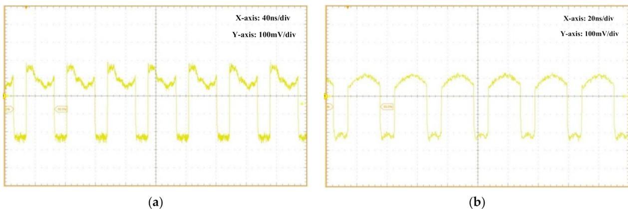
**Figure 10.** Measured output waveforms of the improved programmable frequency divider: (a)  $f_{in} = 12$  GHz,  $n = 648$ ; (b)  $f_{in} = 19$  GHz,  $n = 588$ .
