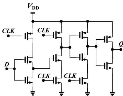
Figure 5. Schematic diagram of a TSPC DFF (DFF1) for an asynchronous divider.
