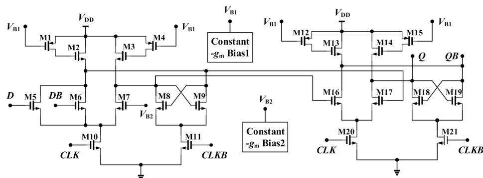
Figure 4. Schematic of the modified DFF based on active inductors integrated with “OR” logic.
