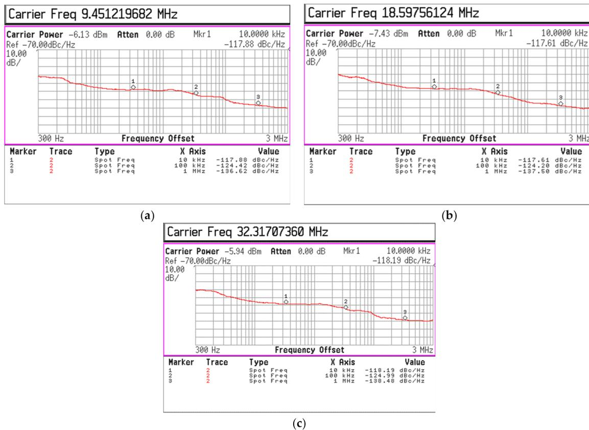
Figure 11. Measured phase noise of the improved programmable integer divider’s output signal: (a)  $f_{in} = 6.2$  GHz,  $n = 656$ , and  $f_{out} = 9.452$  MHz; (b)  $f_{in} = 11.3$  GHz,  $n = 608$ , and  $f_{out} = 18.597$  MHz; and (c)  $f_{in} = 19$  GHz,  $n = 588$ , and  $f_{out} = 32.32$  MHz.
