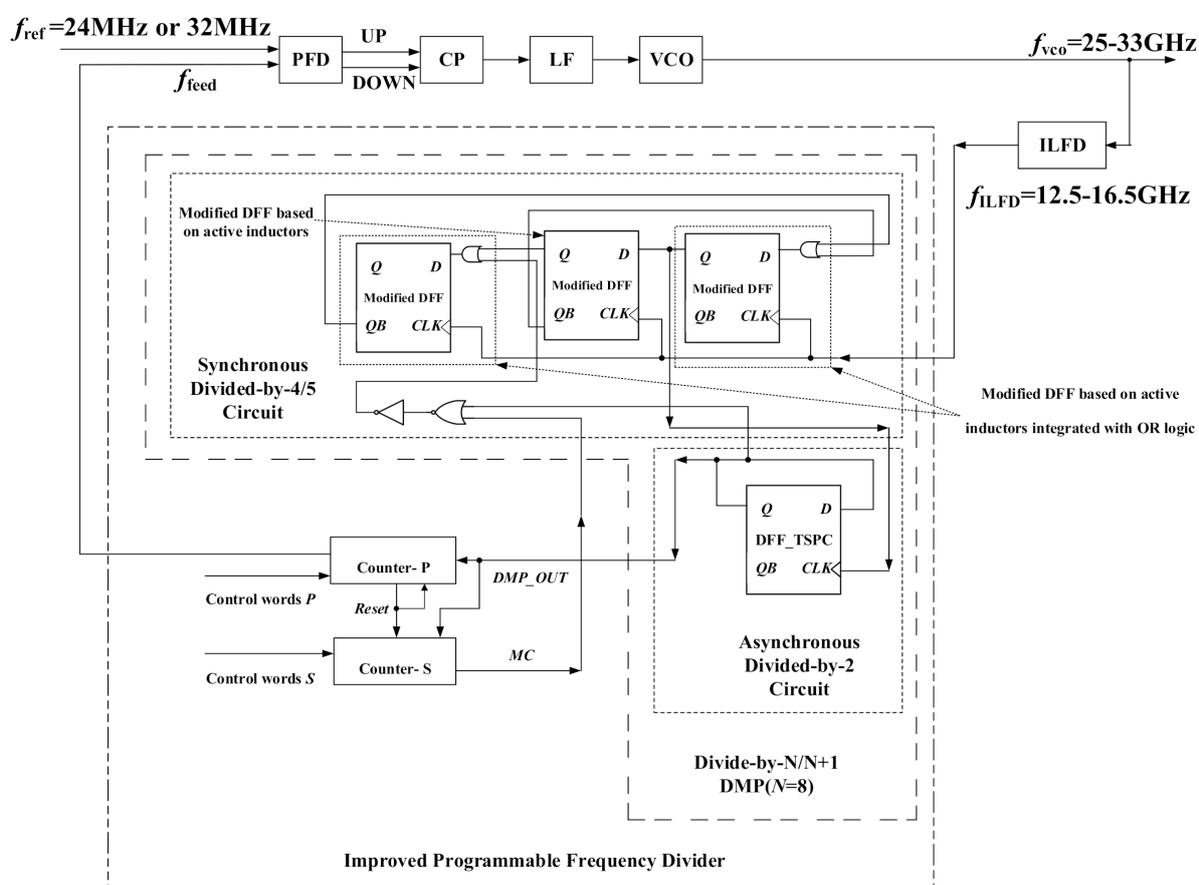
Figure 1. Block diagram of the Ka-band PLL and the improved programmable frequency divider.
