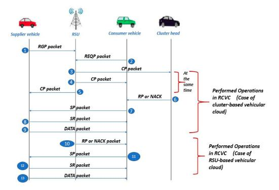
Figure 6. Sequence diagram of packets exchanged by RCVC.
