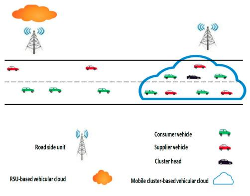
Figure 1. Vehicular cloud types in RSU-aided Cluster-based Vehicular Cloud (RCVC).
