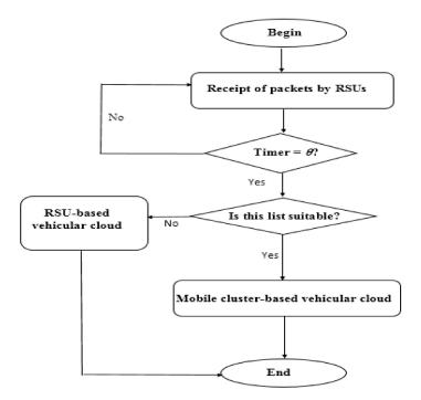
**Figure 3.** Registration and data requests process at the Road Site Unit (RSU) level to enable vehicular clouds.
