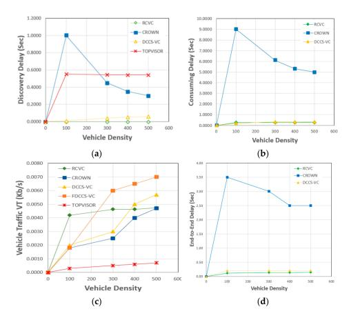
**Figure 10.** Performance evaluation comparisons of RCVC with: (a) CROWN, DCCS-VC and TOPVISOR in terms of Discovery Delay. (b) CROWN and DCCS-VC in terms of Consuming Delay. (c) CROWN, DCCS-VC, FDCCS-VC and TOPVISOR in terms of Vehicle Traffic. (d) CROWN, DCCS-VC in terms of End-to-End Delay.
