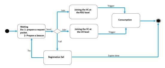
Figure 8. State diagram of the consumer vehicle (CV) object.
