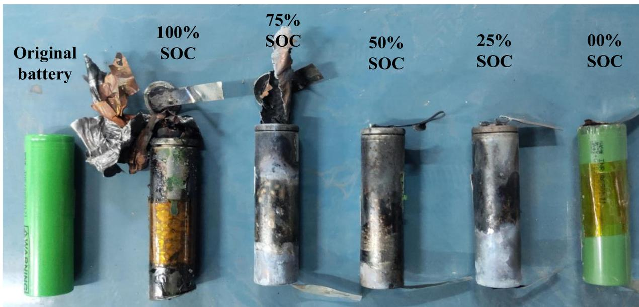
**Figure 8.** The photographs of the sample battery before and after the TR experiment.
