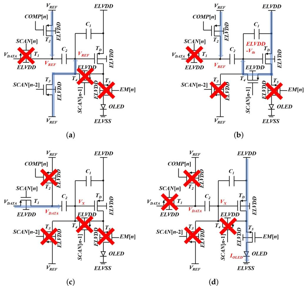
Figure 2. Operation phases of the proposed pixel circuit. (a) Initializing. (b)  $V_{th}$ -sampling. (c) Data programming. (d) Emitting.
