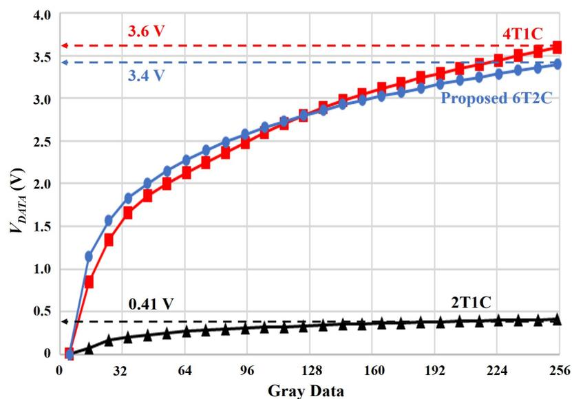
Figure 6. Extended  $V_{DATA}$  ranges of 6T2C and 4T1C circuits, compared to the narrow one of the 2T1C circuit.
