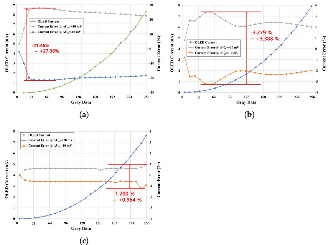
**Figure 7.** OLED currents and current errors over gray data. (a) 2T1C circuit. (b) 4T1C circuit. (c) Proposed 6T2C circuit.
