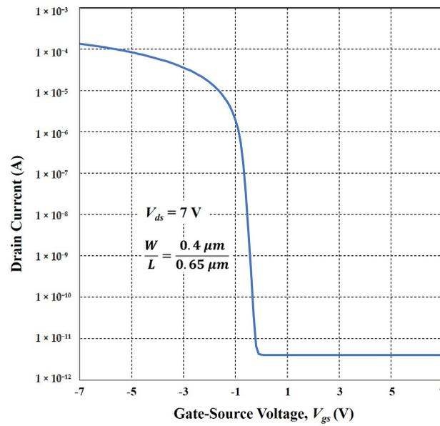
Figure 3. Transfer curve of a PMOS transistor used in the simulation.
