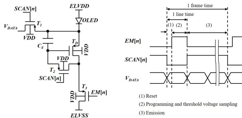
Figure 5. PMOS transistor version of 4T1C pixel circuit and timing diagram.
