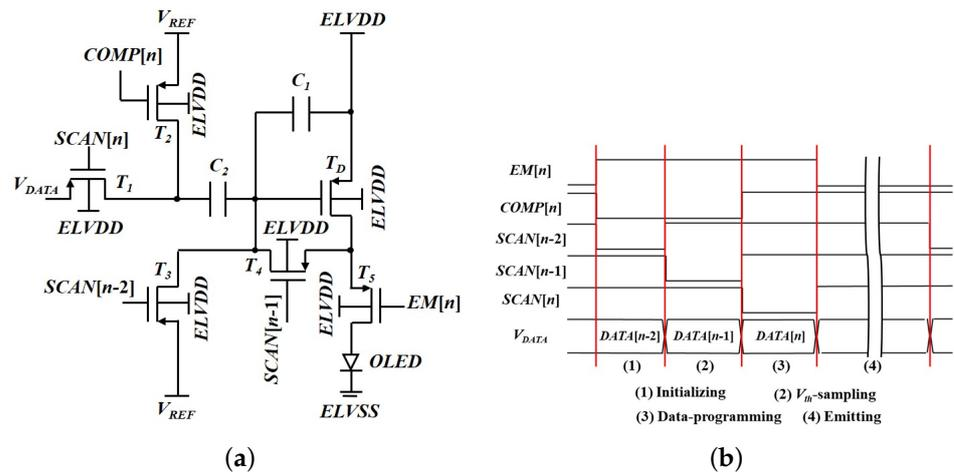
Figure 1. Proposed OLEDoS pixel circuit. (a) Schematic. (b) Timing diagram.
