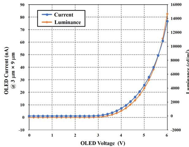
Figure 4. Current and luminance plots of a blue OLED at the sub-pixel area of  $3 \mu\text{m} \times 9 \mu\text{m}$ .
