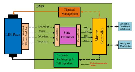
Figure 1. Schematic layout of a generic WBMS.
