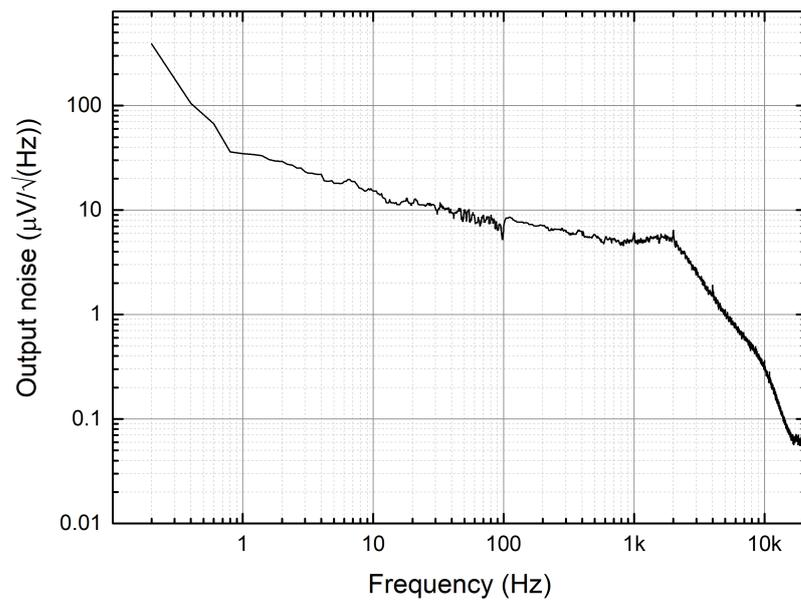
Figure 12. Output noise spectral density. Noise density in the flat region is indicated.
