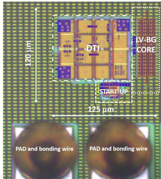
**Figure 8.** Micrograph of the proposed voltage reference with the layout aligned and superimposed in order to show the devices and interconnections that would be otherwise hidden below the planarization dummies. The dimensions and the main blocks are indicated.
