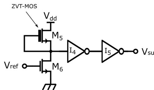
**Figure 7.** Schematic view of the auxiliary LV-comparator.
