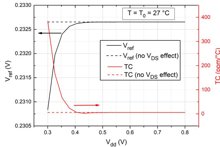
**Figure 5.** Supply voltage dependence of  $V_{ref}$  (at  $T = T_0$ ) and the Temperature Coefficient (TC), considering or neglecting the  $V_{DS}$  effect on the drain current.
