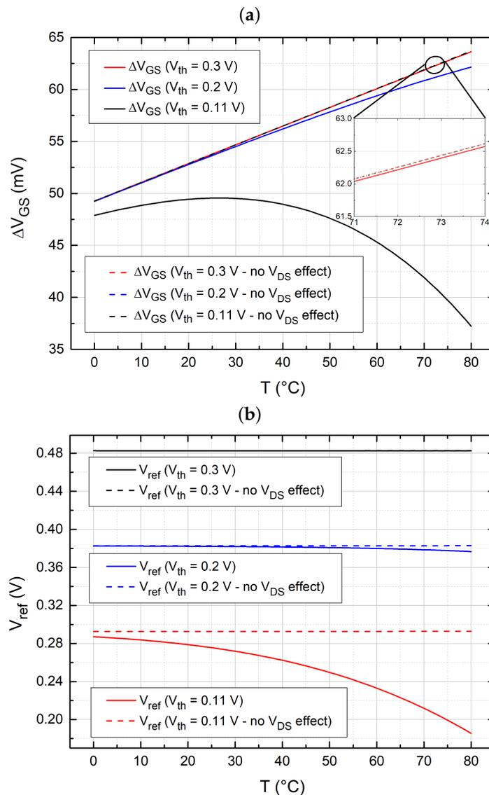
**Figure 2.** Temperature behavior of  $\Delta V_{GS}$  (a) and  $V_{ref}$  (b) in the BG core of Figure 1b, for different values of  $V_{th}$ , considering or neglecting the  $V_{DS}$  effect on the drain current.
