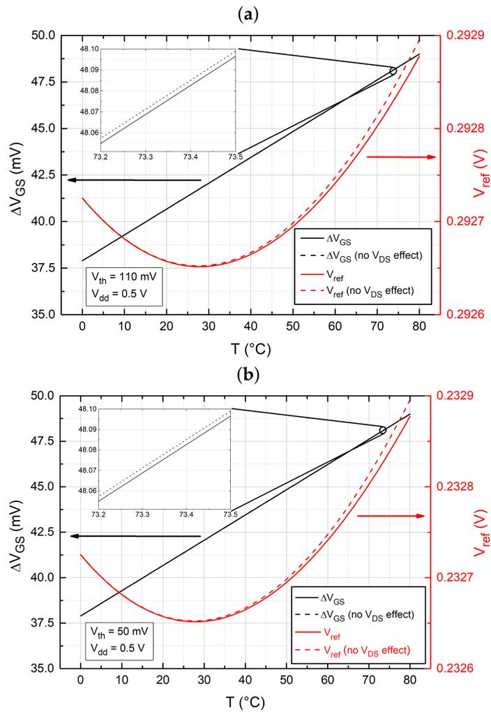
Figure 4. Temperature behavior of  $V_{ref}$  and  $\Delta V_{GS}$  in the BG core of Figure 3a, for  $V_{dd} = 0.5$  V, considering or neglecting the  $V_{DS}$  effect on the drain current, for  $V_{th} = 110$  mV (a) and  $V_{th} = 50$  mV (b).
