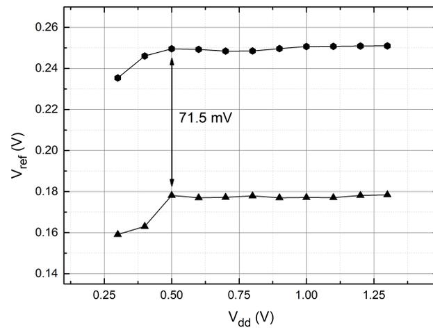
**Figure 9.** Measured output voltage,  $V_{ref}$ , as a function of the power supply at room temperature.
