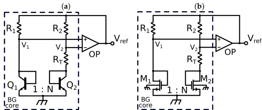
**Figure 1.** Schematic view of (a) the bandgap reference voltage proposed in [15] and (b) its all-MOSFET version.
