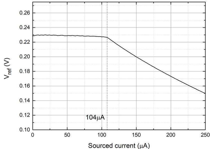
Figure 11. Measured output reference voltage vs. sourced output current.
