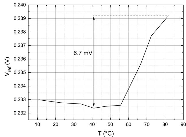
**Figure 10.** Measured temperature dependence of the output voltage in the range 10 °C to 80 °C .
