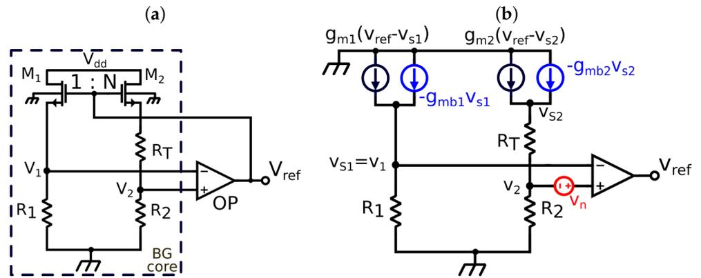
Figure 3. Schematic view of (a) the proposed bandgap reference voltage and (b) its equivalent small signal circuit.
