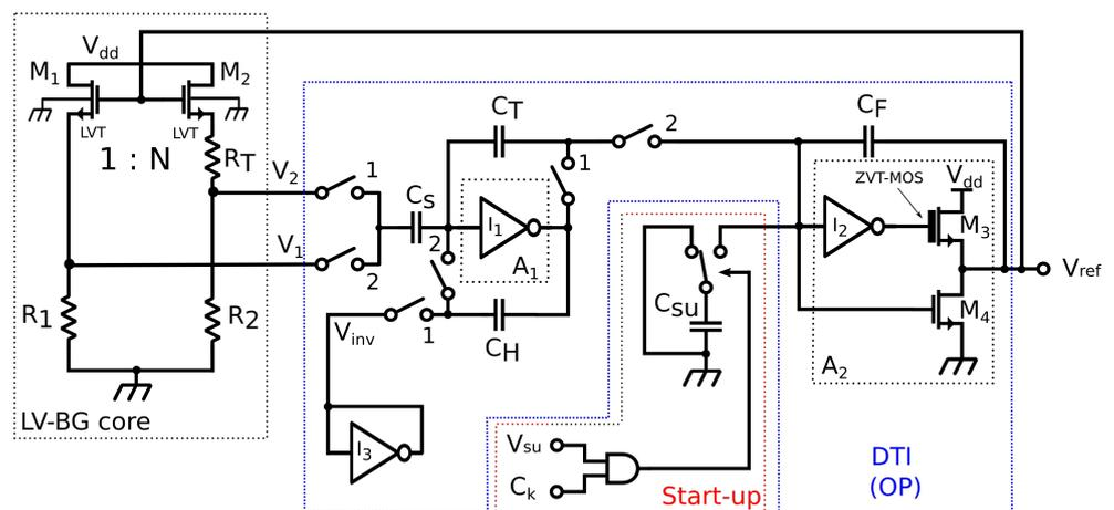
Figure 6. Schematic view of the proposed LV-VR.
