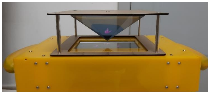
Figure 3. Outward appearance of the holographic imaging system.
