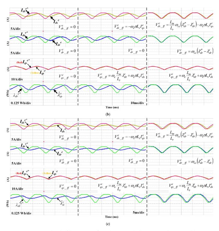
**Figure 11.** Experimental results of the current, rotor flux, and torque controls of a DIFWM according to sinusoidal torque reference: (a) 10 Hz; (b) 50 Hz; (c) 100 Hz.
