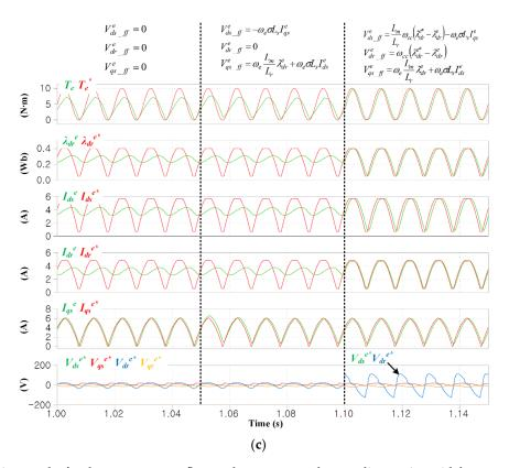
**Figure 6.** Simulation results for the current, rotor flux, and torque controls according to sinusoidal torque reference at a low speed (200 r/min): (a) 10 Hz; (b) 50 Hz; (c) 100 Hz.
