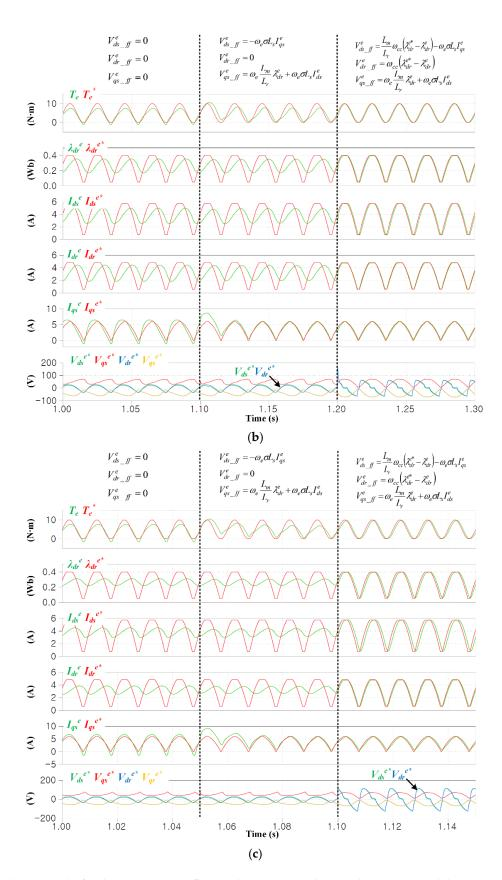
**Figure 7.** Simulation results for the current, rotor flux, and torque controls according to sinusoidal torque reference at the rated speed (1055 r/min): (a) 10 Hz; (b) 50 Hz; (c) 100 Hz.
