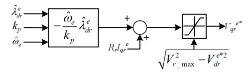
Figure 3. Block diagram of the power distribution control.
