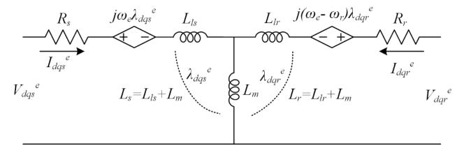
Figure 2. Equivalent model of a DIFWM.
