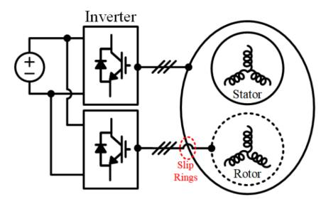
Figure 1. Double inverter-fed wound machine drive system.
