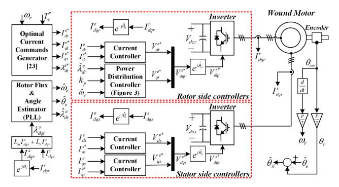
Figure 4. Entire control block diagram of the minimum copper loss control method in a DIFWM [23].
