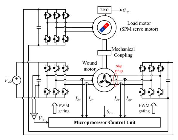
Figure 8. Block diagram of experimental set-up.
