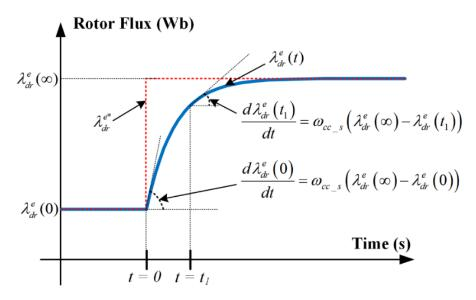
**Figure 5.** Variation of rotor flux according to stepwise command in the proposed control method of a DIFWM.
