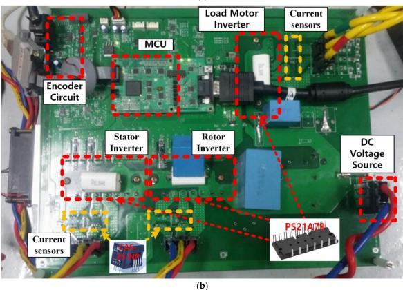
**Figure 9.** Test wound motor and load machine used in experiments: (a) Dynamo set of wound motor and load machine; (b) Inverter set.
