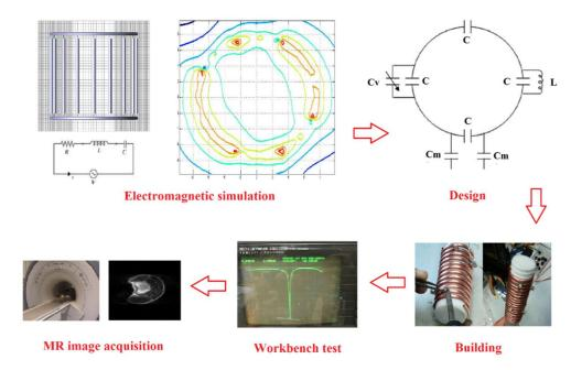
Figure 4. The different phases in the radiofrequency (RF) coil development.
