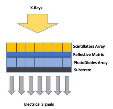
Figure 6. Indirect CT detector.
