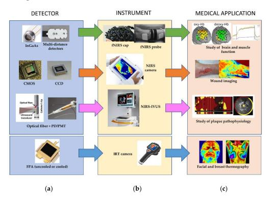
**Figure 2.** Typical detectors (**a**), instruments (**b**), and medical applications (**c**) of near-infrared spectroscopy (NIRS) and infrared thermal (IRT) imaging.
