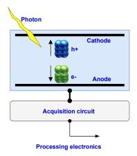
Figure 7. Schematic representation of a CZT-based imaging system.
