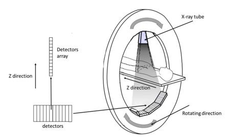
Figure 5. Detectors array design in a multi-slice computed tomography (MSCT) scanner.
