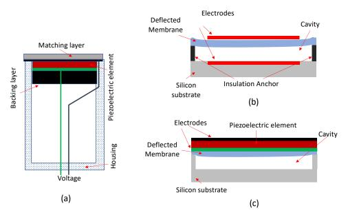
**Figure 1.** Typical schematic view of cross-sectional structures of **(a)** piezoelectric ultrasonic transducers; **(b)** capacitive micromachined ultrasonic transducers (cMUTs) and **(c)** piezoelectric micromachined ultrasonic transducers (pMUTs) transducers.
