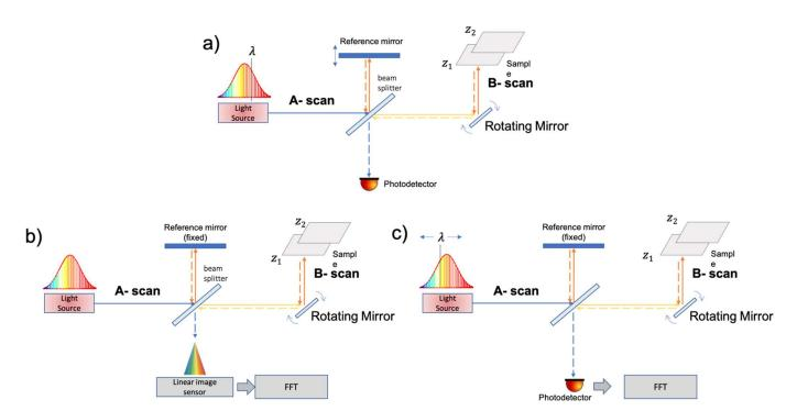
**Figure 3.** Schematic drawing of Michelson interferometer for time domain optical coherence tomography (TD-OCT) (a), spectral-domain OCT (SD-OCT) (b), and swept-source OCT (SS-OCT) (c). In the TD-OCT and SS-OCT, the detector is a photodiode; in SD-OCT, the detector is a spectrometer.
