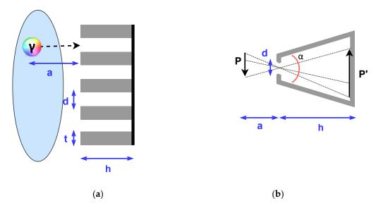
**Figure 8.** Schemes of two typical collimators: parallel hole (**a**) and pinhole (**b**) collimators. The ellipse in (**a**) represents the gamma-ray emitting region. P and P' in (**b**) show how a region of the object is projected and magnified after crossing the collimator (P' > P).
