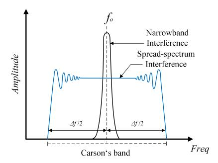
Figure 1. Conventional PWM vs. SSM techniques.
