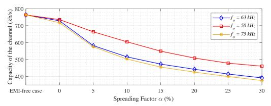
**Figure 12.** The PLC channel capacity in the case of several values of spreading factor with the change in the central switching frequency of SSM.
