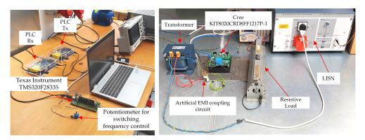
Figure 4. Setup testbed.
