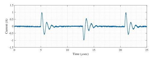
Figure 6. The common mode current due to the parasitic coupling path.
