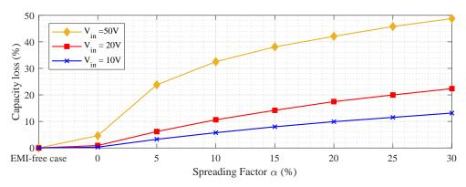
**Figure 10.** The PLC channel capacity loss in the case of several values of spreading factor with the change in input voltage amplitude of the converter.
