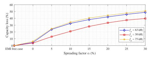
**Figure 13.** The PLC channel capacity loss in the case of several values of spreading factor with the change in the central switching frequency of SSM.
