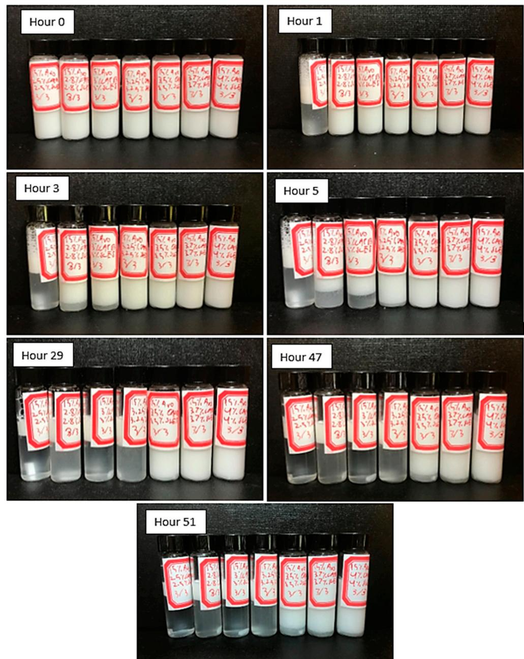
**Figure 2.** 15 wt % avocado oil emulsions' visual stability. From left to right samples are 5 wt %, 5.6 wt %, 6 wt %, 6.5 wt %, 7 wt %, 7.4 wt %, and 8 wt % total CAPB and SLES emulsifier concentrations.
