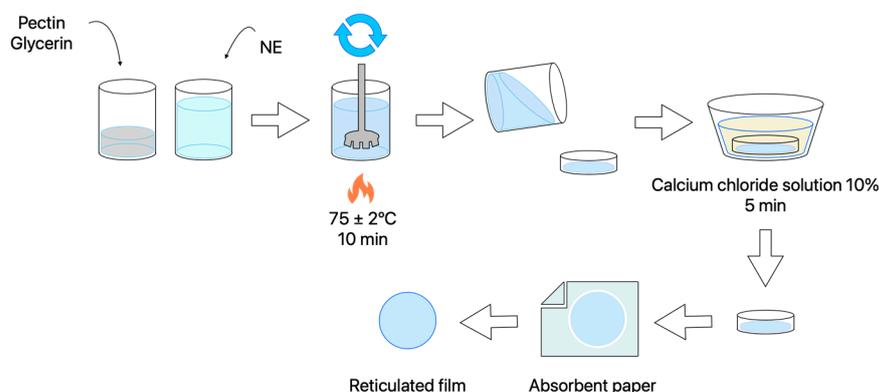
**Figure 1.** Method for preparing pectin/tapioca starch films.
