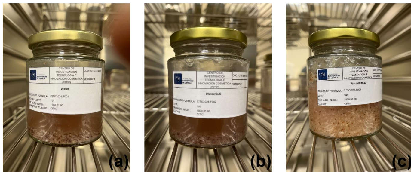
Figure 5. Preliminary tests of sinami seed powder immersed in different substrata. (a) Water; (b) water/sodium laureth sulfate (SLS); (c) water/acrylate C10–30 (C1030).
