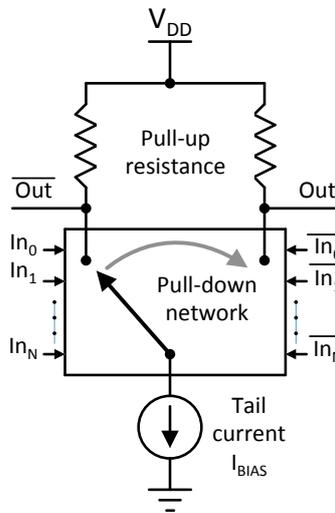
**Figure 3.** Basic MCML gates that share an asymmetric universal MCML gate topology: (a) MCML NAND gate; and (b) MCML NOR gate. The PMOS pull-up gate voltage,  $V_{pbias}$ , is typically connected to ground. The gate voltage,  $V_{nbias}$ , drives the NMOS transistor, providing the tail current.
