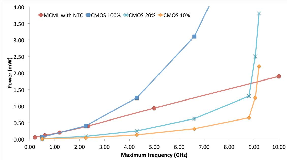
Additionally, above 9 GHz, MCML with NTC is more power efficient than standard CMOS switching at a 10% activity factor. At these frequencies, MCML with NTC is the methodology of choice for general high performance circuits. Activity factors below 25% represent general switching characteristics of typical data paths.
