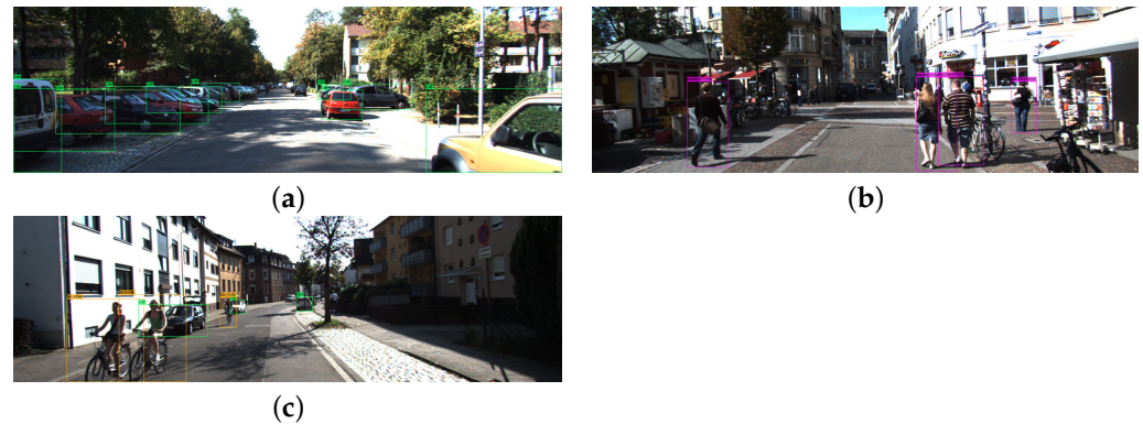
Figure 8. Detecting autonomous vehicle objects using FPGA-based GEMM of YOLOv4 on KITTI dataset. (a) Cars, (b) pedestrians, (c) bicycles.
