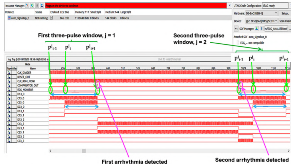
Figure 22. Arrhythmias detection by instrumental analysis performed using the Signal Tap II Logic Analyzer.
