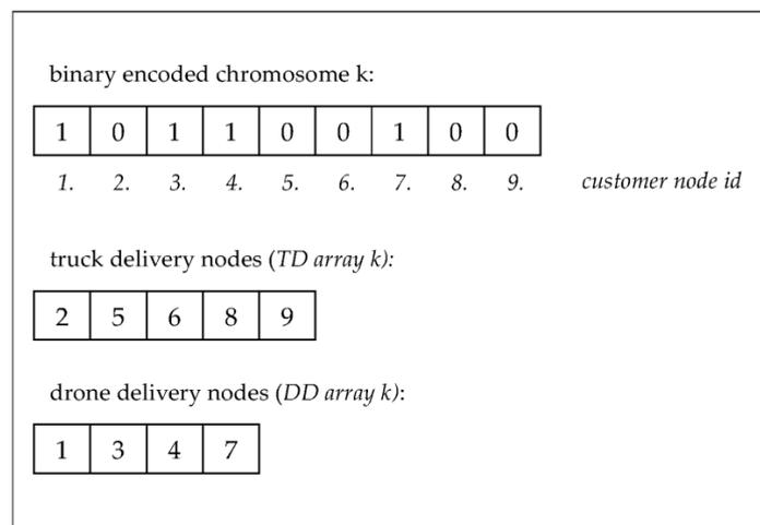
Figure 3. Illustration of a solution representation in GA.
