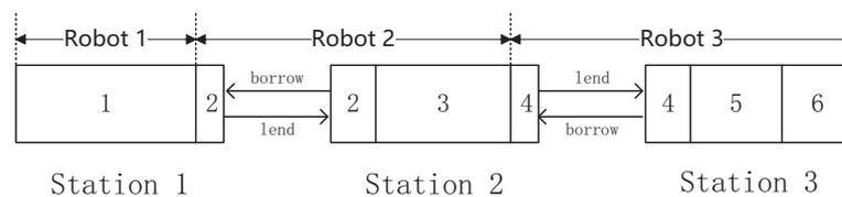
Figure 1. Assembly line with cross-station task design.
