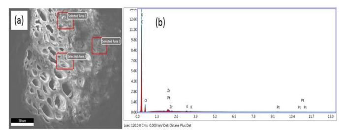
**Figure 5.** (a) SEM micrograph of biochar and (b) EDX graph of biochar after arsenic adsorption at optimized conditions.
