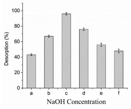
**Figure 7.** %Desorption of arsenic from BCXZM composite after optimized experiment. Note: (a) 0 M, (b) 0.01 M, (c) 0.05 M, (d) 0.5 (e) 0.1 M and (f) 1 M NaOH; Mean  $\pm$  Standard deviation (n = 2).
