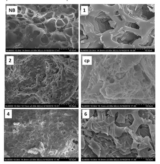
**Figure 3.** SEM micrographs of the bacterial biofilm formation on multifunction biochar at different pH values and arsenic concentrations. Note: NB: native biochar, 1, 2, 4, 6 and cp: correspond to the experimental conditions according to Table 1.
