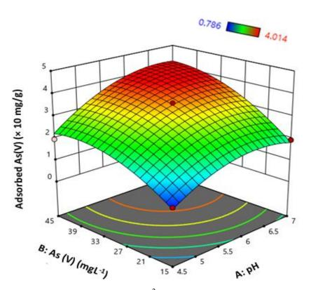
Figure 2. Response surface for (CCD)2<sup>2</sup> experiment of Adsorbed As(V) by BCXZM composite.
