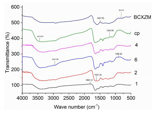
**Figure 6.** FTIR spectra of the native biochar and BCXZM composites after As(V) adsorption. Note: 1, 2, 4, 6 and cp correspond to the experimental conditions according to Table 1.
