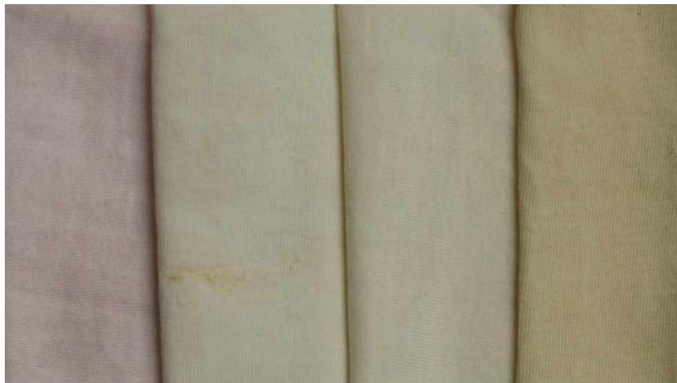
Figure 11. Dyed samples, from left; untreated, salt dyed, mordanted, and cationized.
