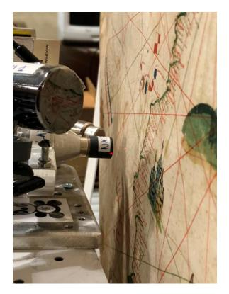
Figure 3. In situ XRF analysis of the map.
