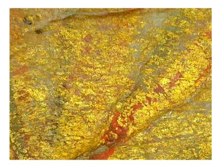
**Figure 9.** Gilded wind rose observed under digital Dino microscope. Gold foil was placed on a transparent *mixtion* (reproduced with permission from the AGI).
