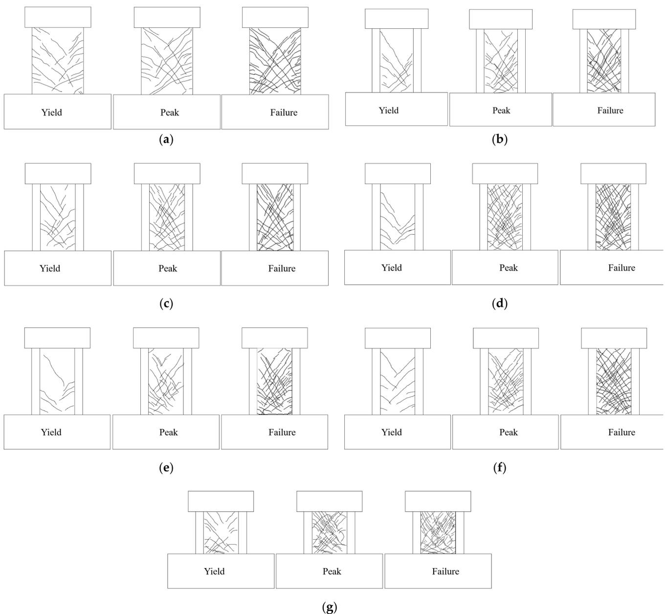
**Figure 4.** The failure process of all specimens: (a) RHC-0; (b) CFST-1; (c) CFST-2; (d) CFST-3; (e) CFST-4; (f) CFST-5; (g) CFST-6.
