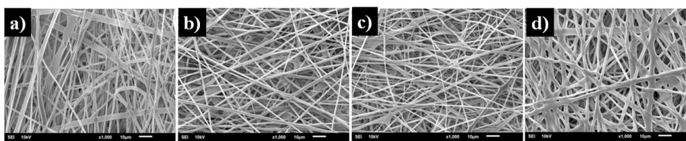
**Figure 3.** Electrospun gelatin nanofibers with various concentrations of crude ethanol extract of *Curcuma comosa* Roxb.rhizome powder: (a) 1%, (b) 5%, (c) 10%, and (d) 15% (w/v) in acetic acid/H<sub>2</sub>O (9:1 (v/v)).
