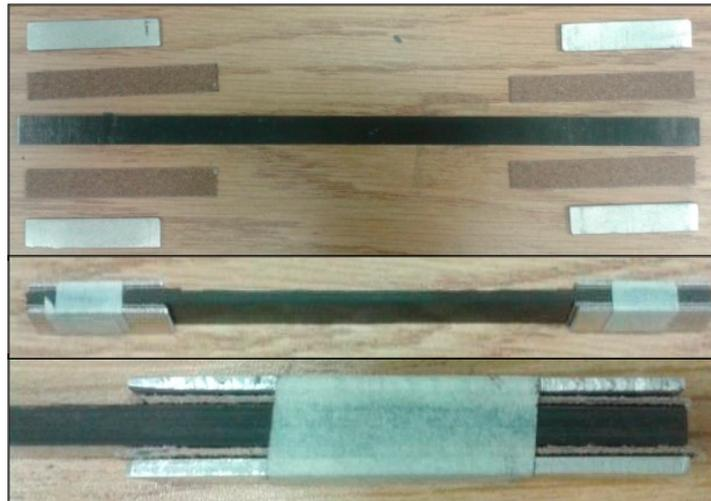
**Figure 6.** Sample with sandpaper and aluminium tabs.
