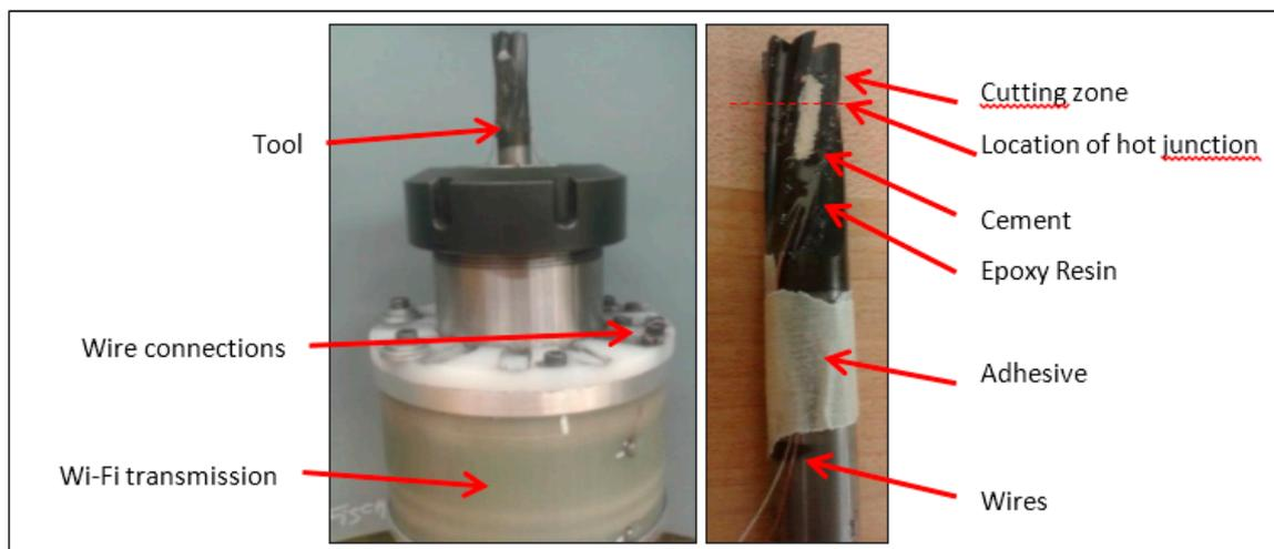
**Figure 4.** Mandrel and new tool equipped with thermocouple.
