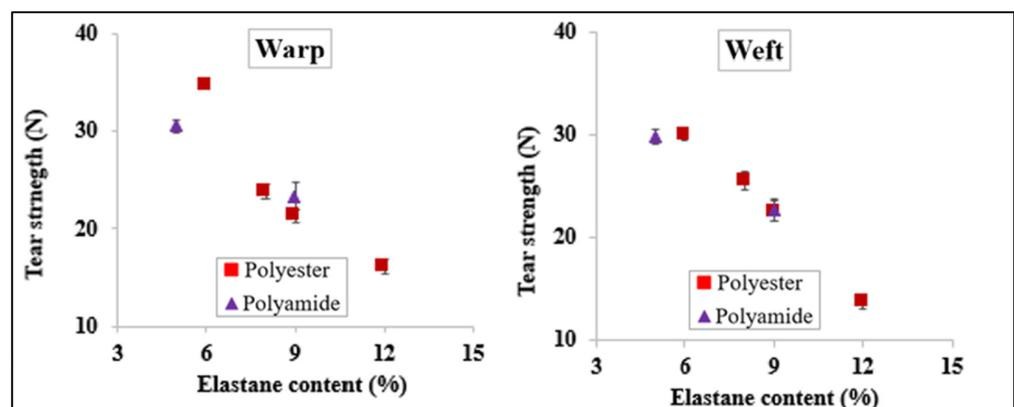
**Figure 9.** Variation of the fabric tear strength as a function of the elastane content in both directions.
