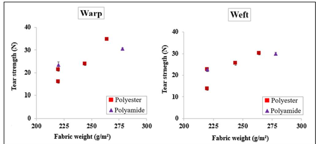
**Figure 8.** Variation of the fabric tear strength as a function of the fabric weight in both directions.
