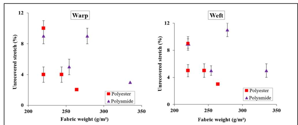
**Figure 10.** Variation of the fabric unrecovered stretch as a function of the fabric weight in both directions.
