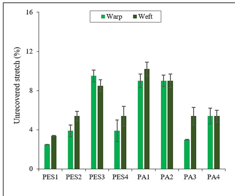
Figure 5. Unrecovered stretch of Fabric PES1 to PES4 and PA1 to PA4 in both directions.
