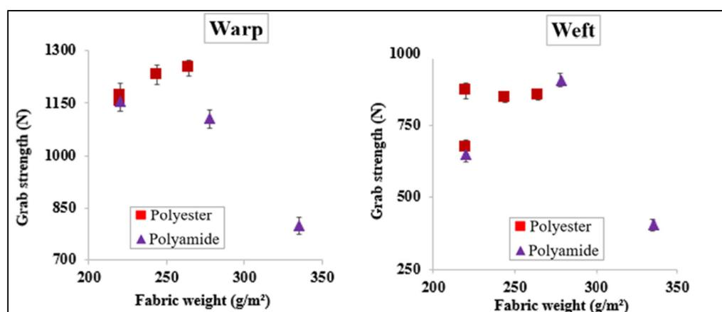
Figure 6. Variation of the fabric grab strength as a function of the fabric weight in both directions.
