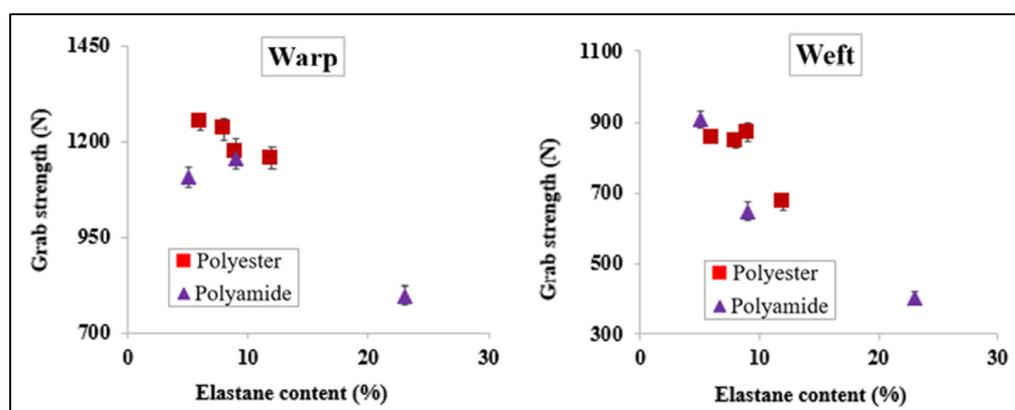
Figure 7. Variation of the fabric grab strength as a function of the elastane content in both directions.
