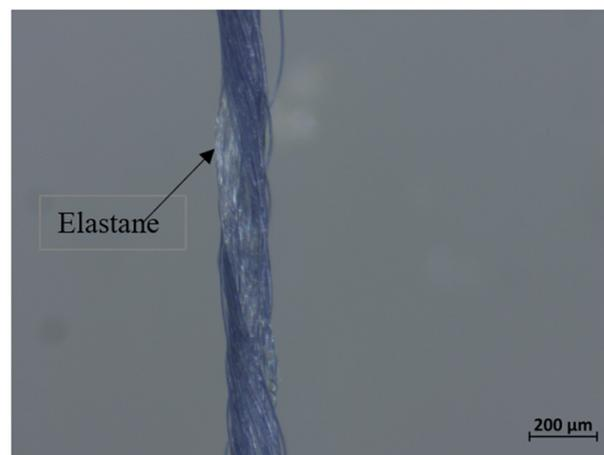
**Figure 1.** Microscopic image of a stretched strand of the weft yarn in PA4 at 2.5× magnification.
