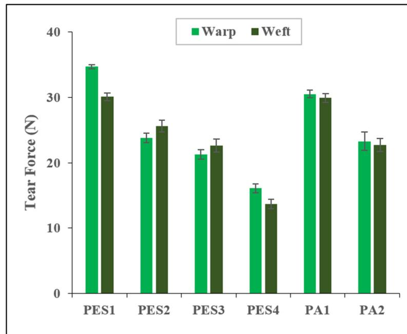
Figure 4. Tear strength of Fabric PES1 to PES4, PA1, and PA2 in both directions.
