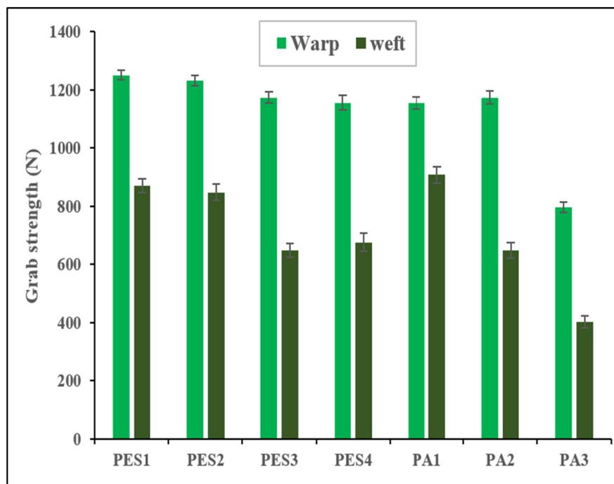
**Figure 3.** Grab strength of Fabric PES1–PES4 and PA1–PA3 in both directions.
