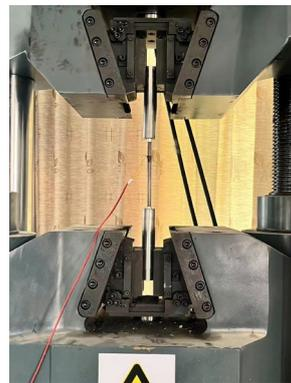
Figure 4. Tensile testing for CFRP tendon.
