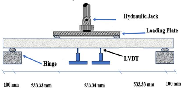
Figure 12. Test setup.
