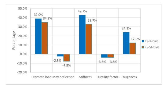
**Figure 21.** Percentage of the impact of CFRP form (rope and strip) on the characteristics of the load-deflection curve at 20 cm.
