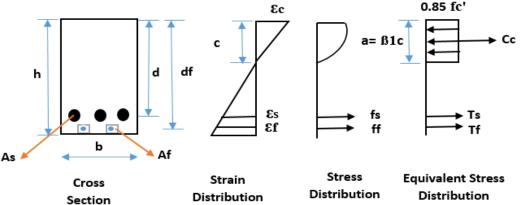
**Figure 22.** Stress and strain compatibility of concrete rectangular cross sections strengthened by NSM-CFRP under flexural capacity.
