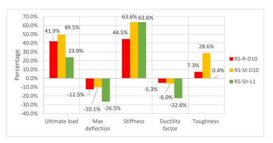
**Figure 20.** Percentage of the impact of CFRP form (rope, strip, and sheet) on the characteristics of the load-deflection curve at 10 cm.
