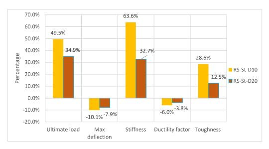
**Figure 18.** Percentage of the impact of the spacing between the strips on the characteristics of the load-deflection curve.
