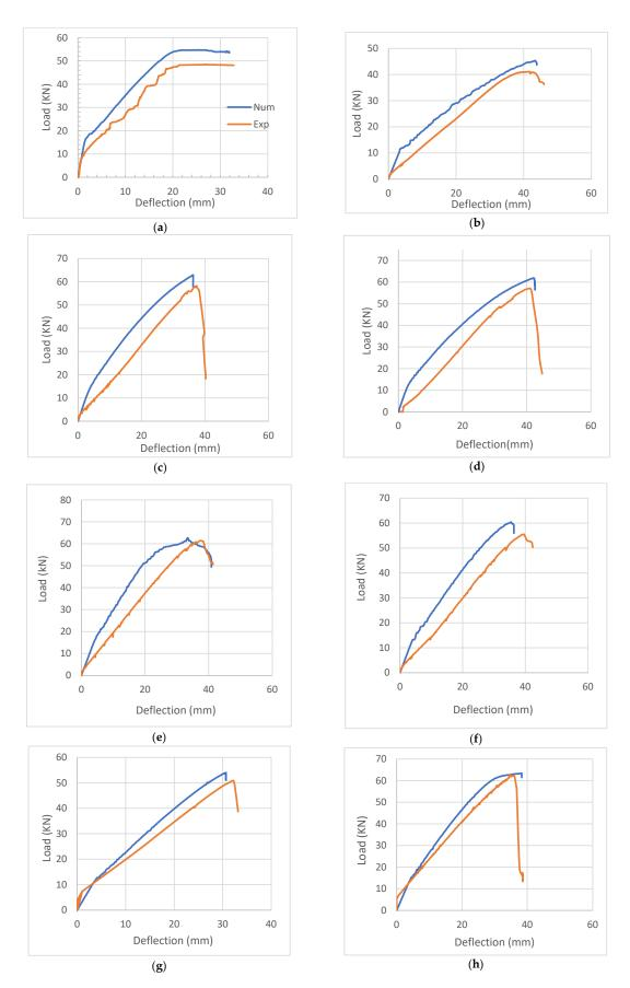
**Figure 24.** Load-deflection curve for experimental vs. numerical results: (**a**) CS avg-N; (**b**) CS3-TS; (**c**) RS-R-D10; (**d**) RS-R-D20; (**e**) RS-St-D10; (**f**) RS-St-D20; (**g**) RS-Sh-L1; (**h**) RS-Sh-L2.
