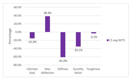
Figure 16. Percentage of the impact of thermal shock on the characteristics of the load-deflection curve.
