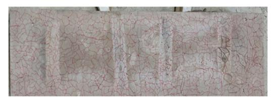
Figure 7. Crack developed by thermal shock.
