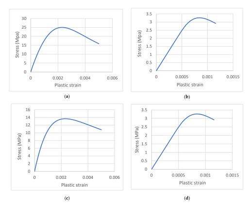
**Figure 23.** Stress–strain diagram: (**a**) compressive curve for unheated slab; (**b**) tensile curve for unheated slab; (**c**) compressive curve for heated slab; (**d**) tensile curve for heated slab.
