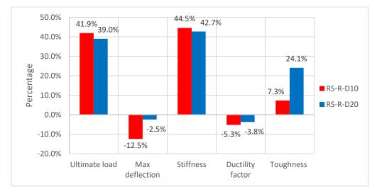
**Figure 17.** Percentage of the impact of the spacing between the ropes on the characteristics of the load-deflection curve.
