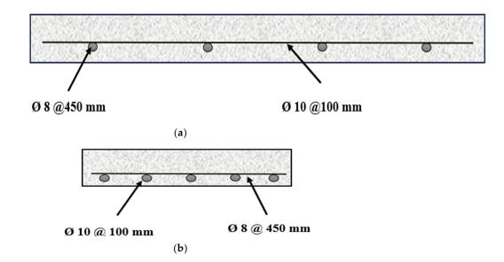
Figure 4. Reinforcement detail: (a) longitudinal direction; (b) transverse direction.
