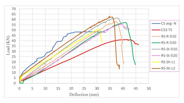
The maximum improvement in ultimate load was 53.4%, achieved using two sheets, while the minimum improvement was 23.9%, observed with using one sheet. Furthermore, the ultimate load of all slabs was restored after being exposed to thermal shock.
