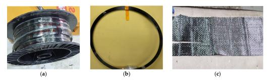
Figure 1. CFRP materials: (a) rope; (b) strip; (c) sheet.
