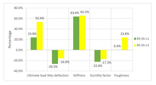
**Figure 19.** Percentage of the impact of the number of sheet layers on the characteristics of the load-deflection curve.
