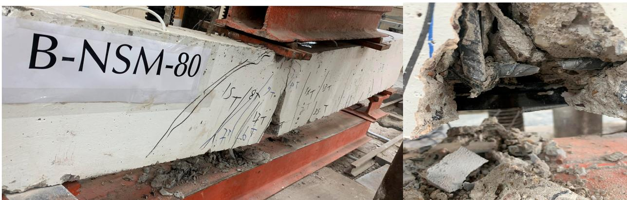
Figure 19. Crack pattern at failure of specimen B-NSM-80.
