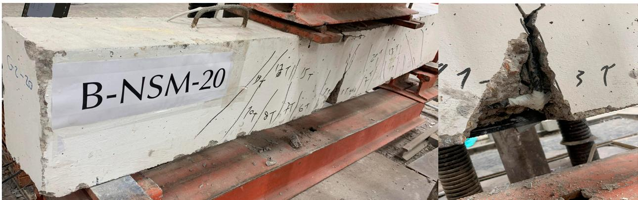
Figure 16. Crack pattern at failure of specimen B-NSM-20.
