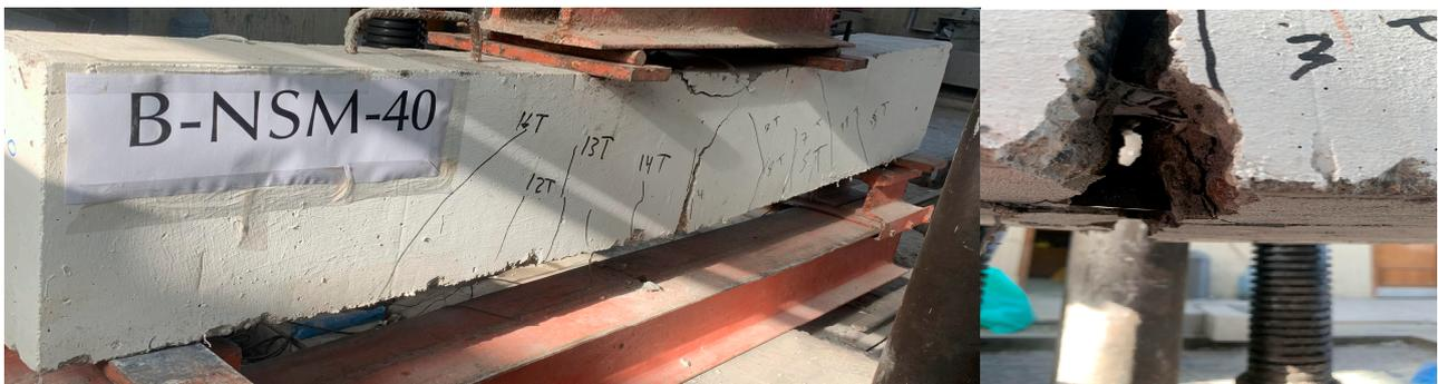
Figure 17. Crack pattern at failure of specimen B-NSM-40.
