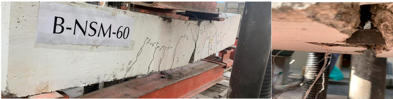
Figure 18. Crack pattern at failure of specimen B-NSM-60.
