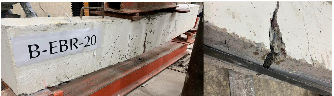
Figure 12. Crack pattern at the failure of specimen B-EBR-20.
