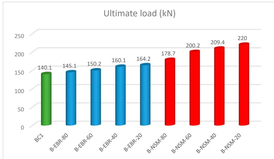
Figure 20. Ultimate load for all beams.
