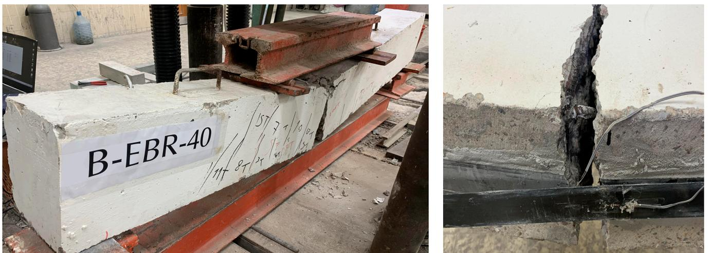
Figure 13. Crack pattern at failure of specimen B-EBR-40.
