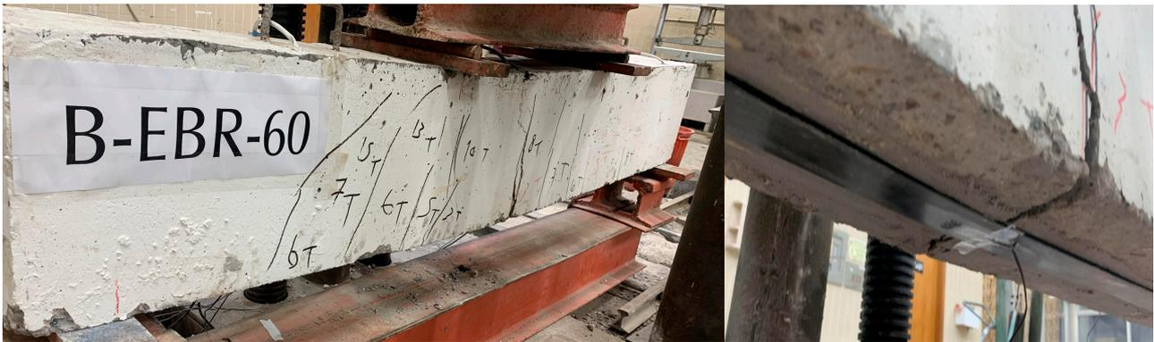
Figure 14. Crack pattern at failure of specimen B-EBR-60.
