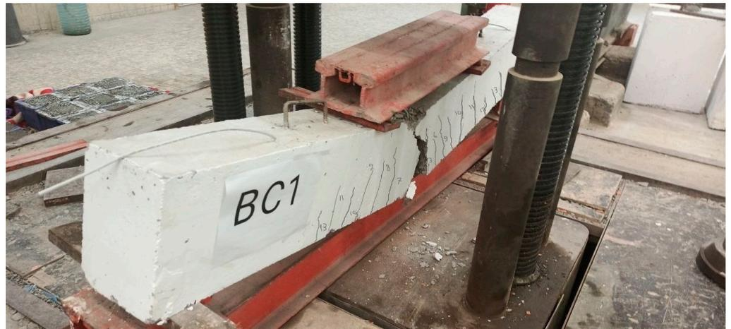
Figure 11. Crack pattern at failure of specimen BC1.
