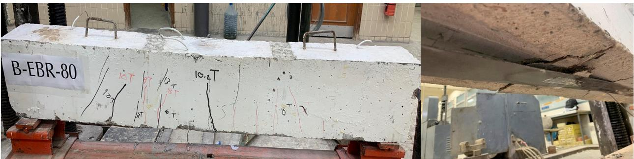
Figure 15. Crack pattern at failure of specimen B-EBR-80.
