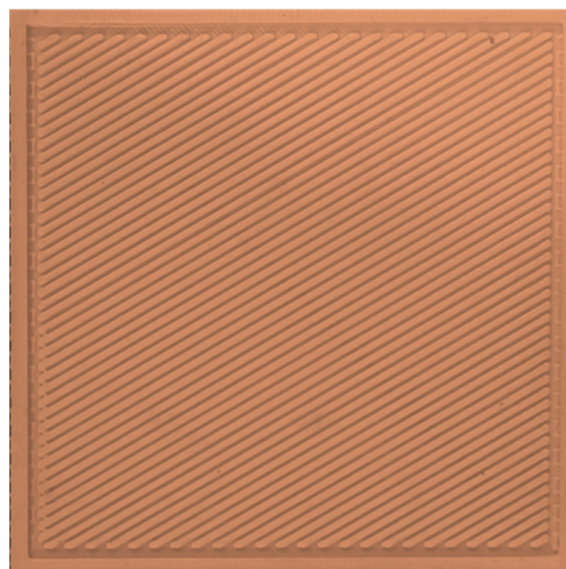
Figure 1. A representative 3D printed mould with 30° fiber alignment.
