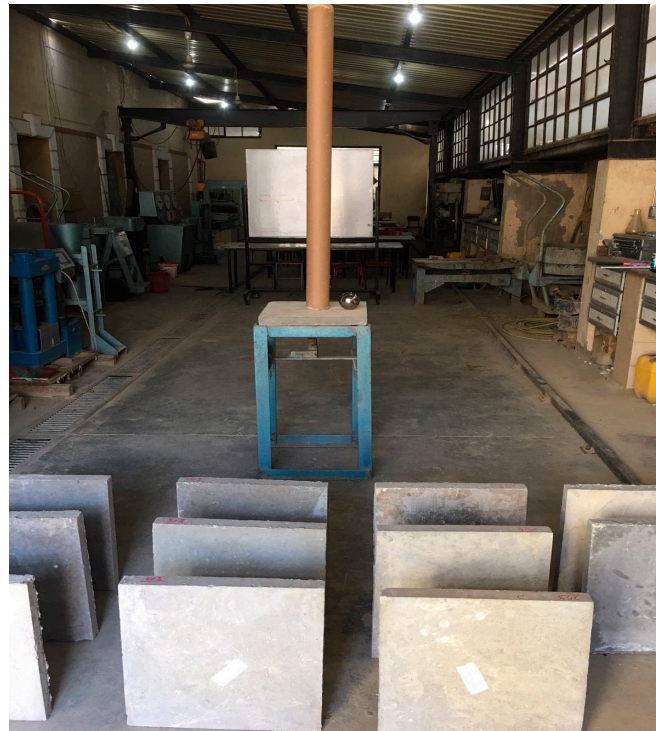
Figure 1. Drop weight impact test equipment.
